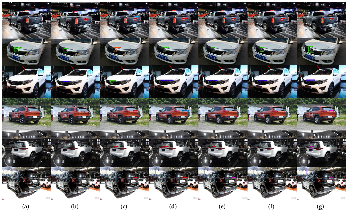
Figure 13. Comparison of detection effect of each detection model: (a) example of detection effect of SSD; (b) example of detection effect of RetinaNet; (c) example of detection effect of Free Anchor; (d) example of detection effect of Centernet; (e) example of detection effect of EfficientDet_d2; (f) example of detection effect of YOLOv5; (g) example of detection effect of My Model.
