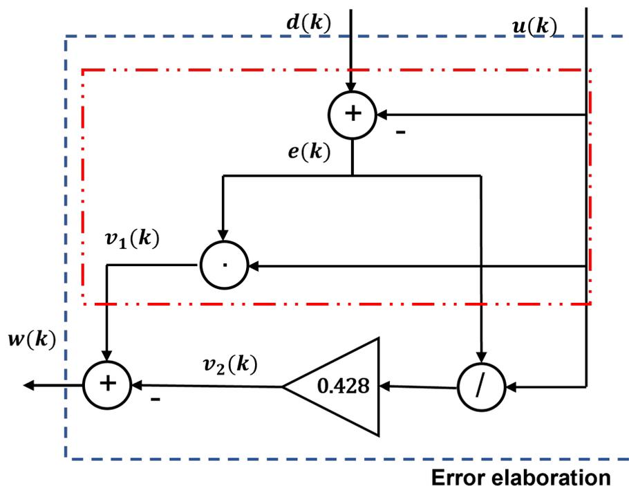
**Figure 6.** The block that processes the difference between the input and the output of the slicer allowing cancellation of the residual ISI and gain error in blue (in red the non-robust to ISI and gain elaboration block).
