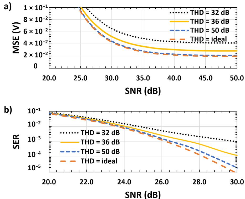
Figure 1. (a) MSE and (b) SER with the varying of SNR for various THD [8].
