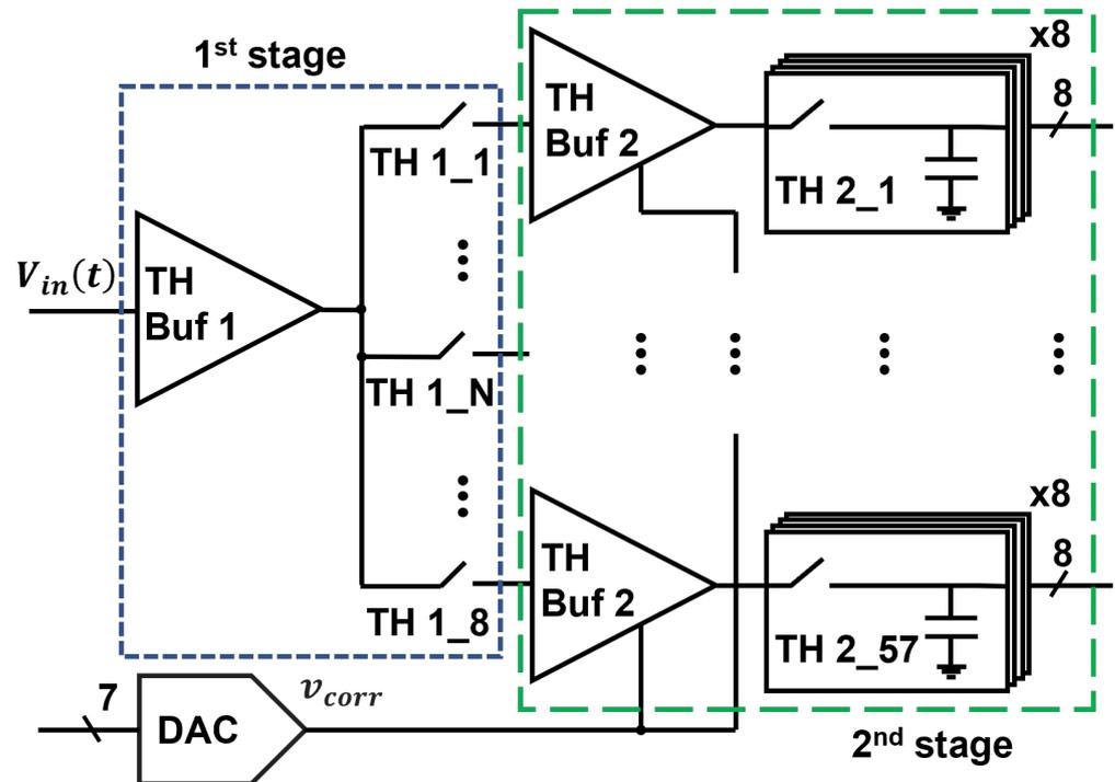
**Figure 2.** Block diagram of a 64 TI-TH circuit with in blue the first stage sampler and in green the second state, using a DAC for the second-stage buffer bias voltage control [8].
