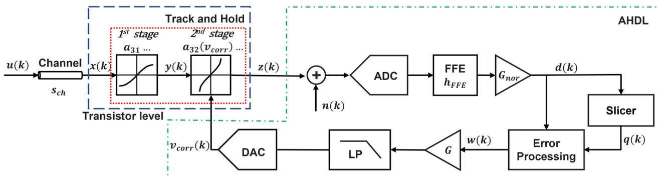
Figure 5. PAM-8 RX using the calibration loop with the transistor level components in blue and the Verilog-A model in green.
