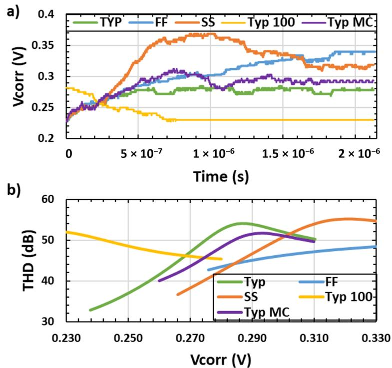
Figure 7. (a) Settling of the  $v_{corr}$  overtime during the calibration of the system and (b) the THD of the TH circuit across different values of  $v_{corr}$  for three different PVT conditions, one MC point, and one after a temperature step (the plot stops at  $v_{corr} = 0.33$  V due to the linearity saturation (FF) for higher values).
