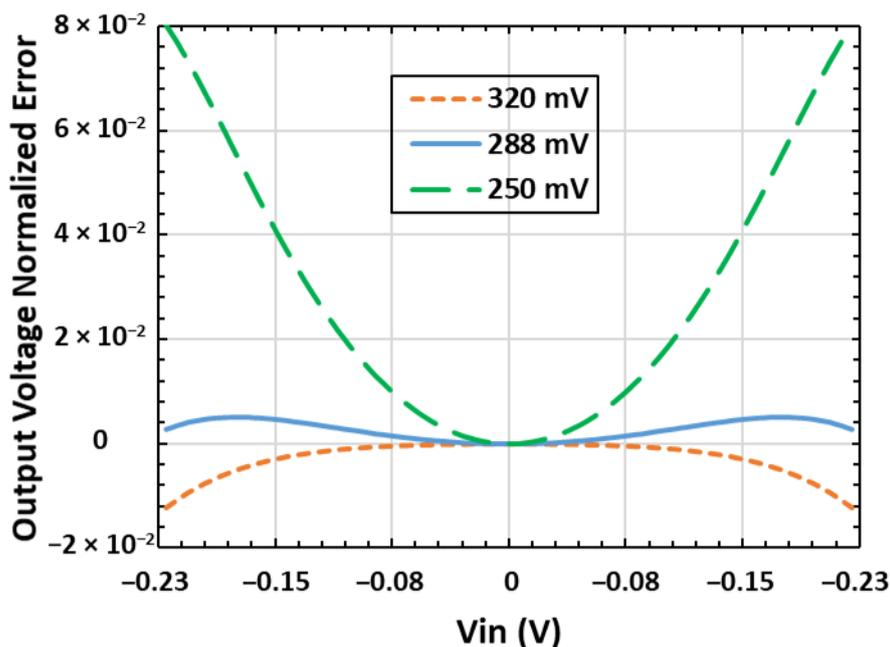
Figure 4. The  $\epsilon_r$  with the varying of the large-signal differential input for various bias voltages  $v_{corr}$  [8].
