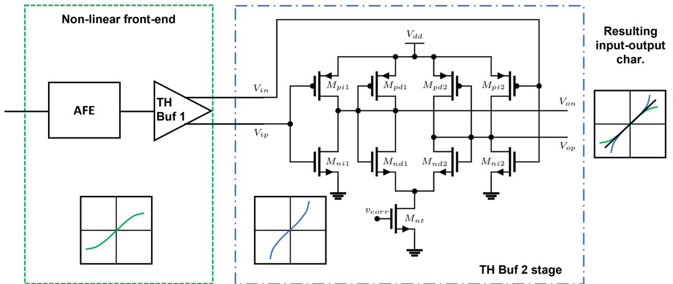
**Figure 3.** Second-stage TH buffer in blue with its distortion contribution compensating for the previous stages non-linear block in green [8].
