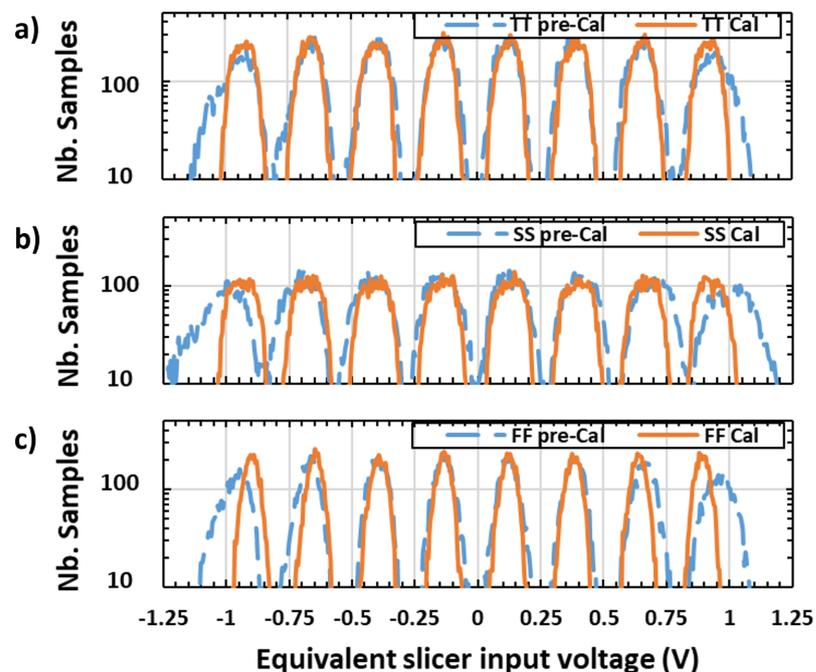
Figure 8. Histograms of the reconstructed signals at the slicer input before and after the linearity calibration for (a) Typical, (b) SS, and (c) FF corner.
