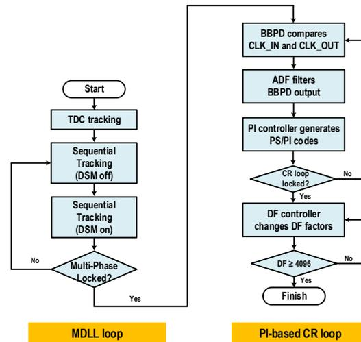
Figure 4. Flowchart illustrating the dual-loop operation of the proposed all-digital DJA.
