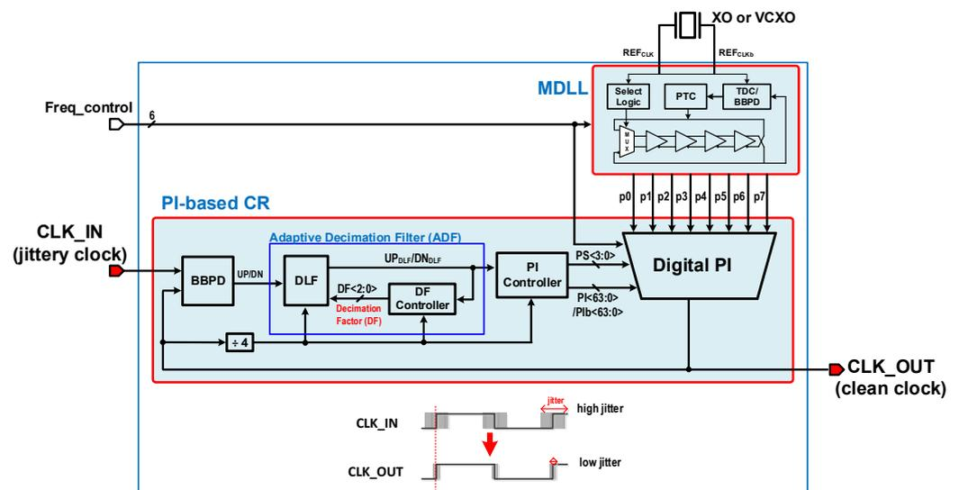
Figure 3. Proposed all-digital dual-loop jitter attenuator (DJA) architecture.
