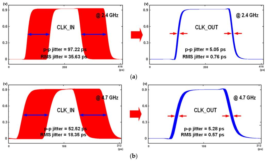
Figure 12. Post-layout simulation results of the proposed DJA showing input and output clock jitter eye diagram at (a) 2.4 GHz and (b) 4.7 GHz.
