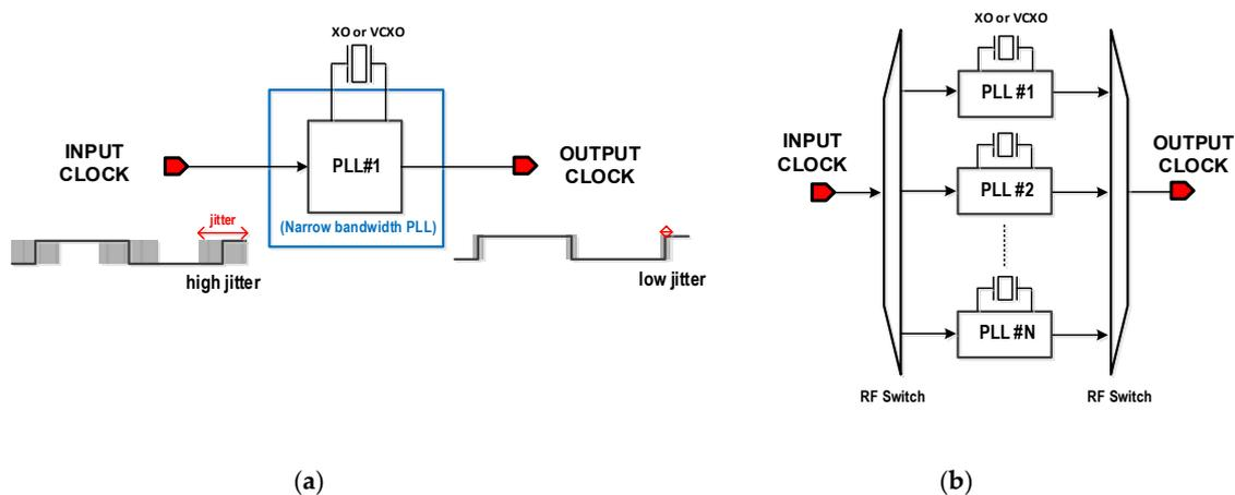
Figure 2. (a) Conventional PLL-based clock jitter attenuator. (b) Simplified block diagram of a wide-range jitter attenuator architecture using multiple PLLs.
