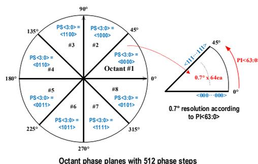
Figure 7. Phase interpolation method of the proposed 9-bit PI with 512 ( $=2^9$ ) steps.
