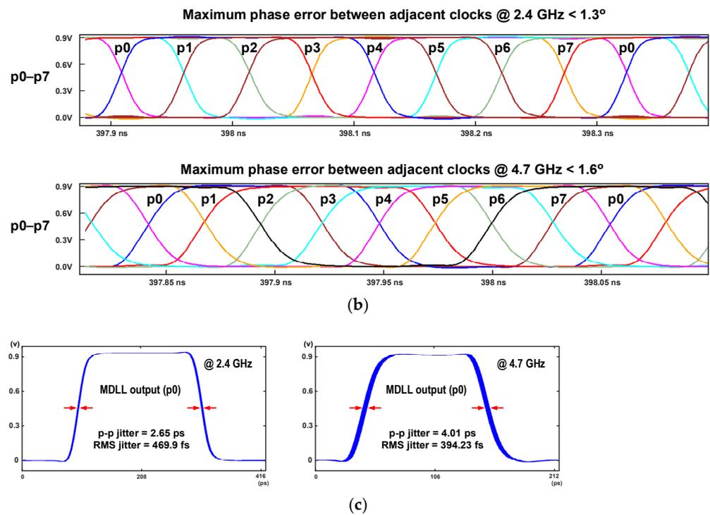
**Figure 5.** (a) Proposed low-jitter eight-phase all-digital MDLL, (b) eight-phase output clocks of the MDLL, and (c) post-layout-based jitter simulation performance of the proposed all-digital MDLL.
