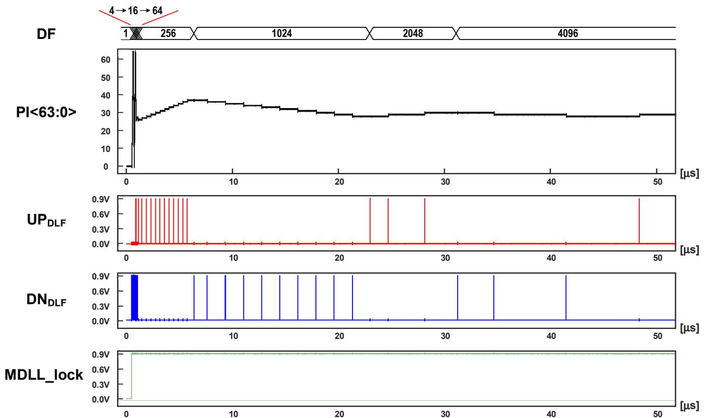
Figure 10. Post-layout simulated locking process of proposed DJA.
