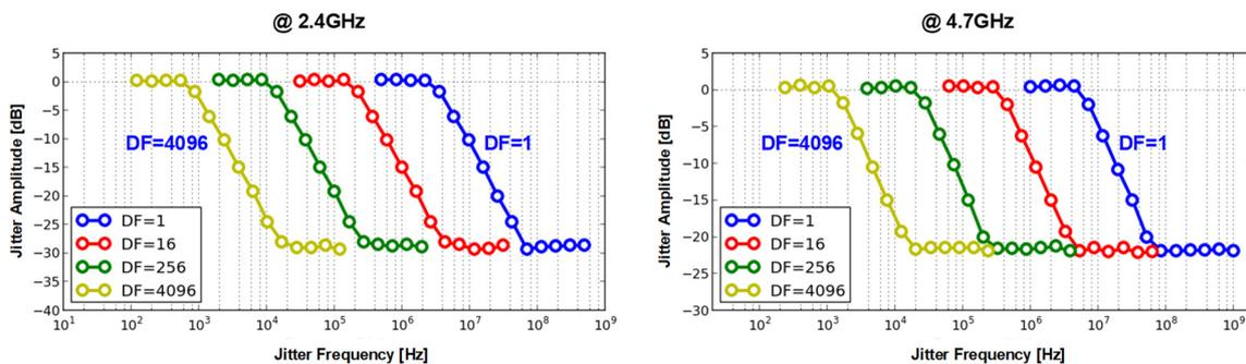
Figure 11. Simulated jitter transfer simulation results at 2.4 GHz and 4.7 GHz.
