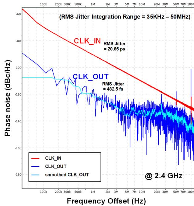
Figure 13. Post-layout-based phase noise simulation plots at 2.4 GHz output frequency.
