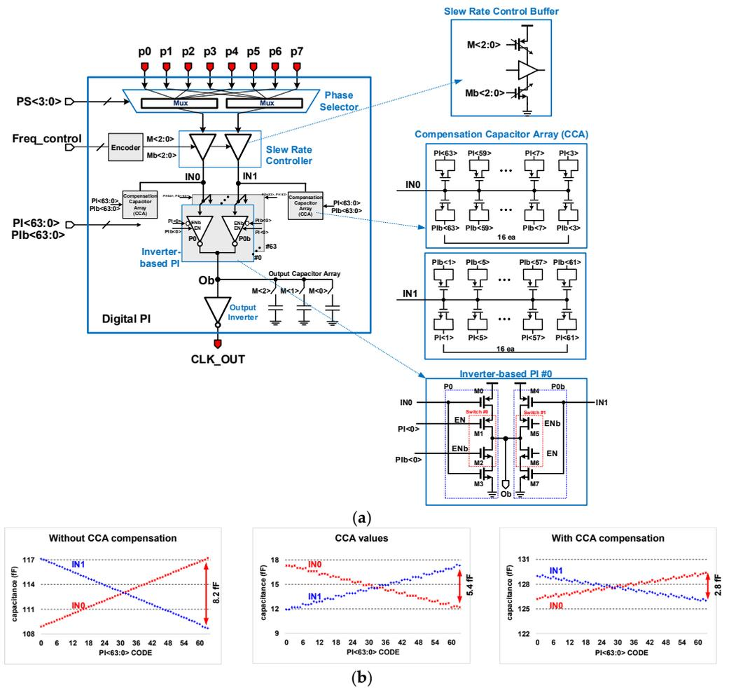
Figure 6. (a) Proposed digital PI. (b) N0/N1 node capacitance compensation using the compensation capacitor array (CCA).
