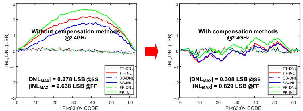
Figure 8. Post-layout corner simulation results of the proposed digital PI showing the INL and DNL of the PI, with and without the proposed compensation methods.
