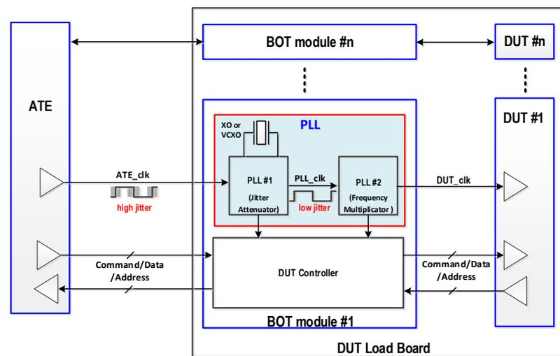
Figure 1. Simplified block diagram of a BOT-based parallel multi-DUT test system.
