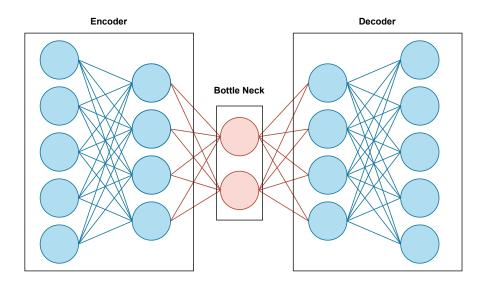
Figure 1. Autoencoder architecture.
