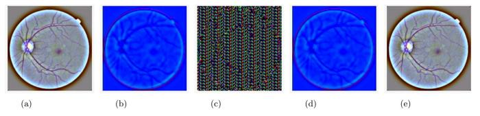
**Figure 6.** The image changes during its journey from receiver to sender: (**a**) original image, (**b**) image outputted from the encoder (sender's side), (**c**) image after encryption (sender's side), (**d**) image after decryption (receiver's side), (**e**) image outputted from the decoder (receiver's side).
