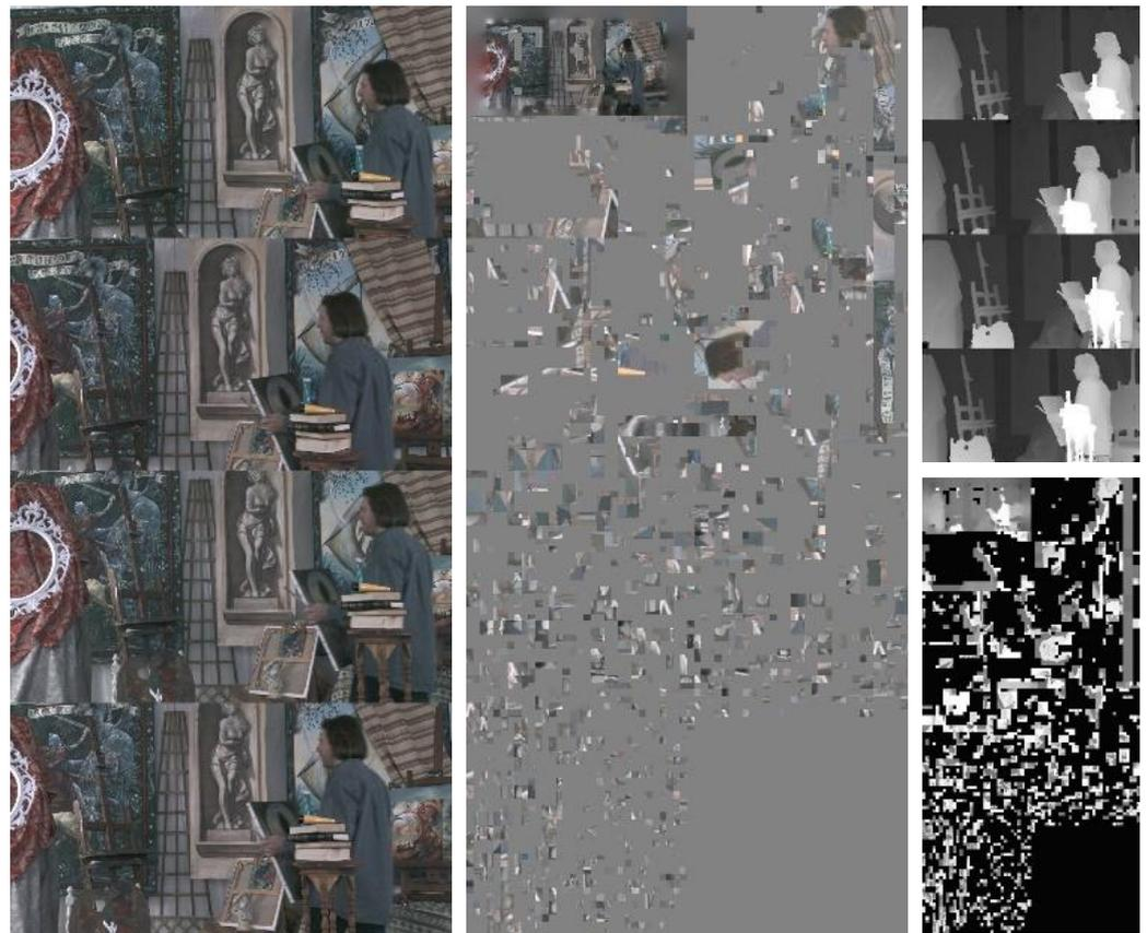
**Figure 1.** Simplified MPEG Immersive Video coding scheme; input data:  $N$  input views, corresponding depth maps, and camera parameters (intrinsic and extrinsic); MIV encoder output—metadata and 4 video streams, including two texture atlases with corresponding depth atlases; each video stream is independently encoded using basic HEVC encoder.
