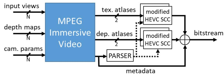
**Figure 3.** Simplified MPEG immersive video coding scheme with modified HEVC SCC encoder controlled by MIV metadata; input data:  $N$  input views, corresponding depth maps, and camera parameters (intrinsic and extrinsic); MIV encoder output—metadata and 4 video streams, including two texture atlases with corresponding depth atlases; each video stream is independently encoded using modified HEVC SCC encoder, encoding parameters (e.g., QP) are controlled by MIV metadata.
