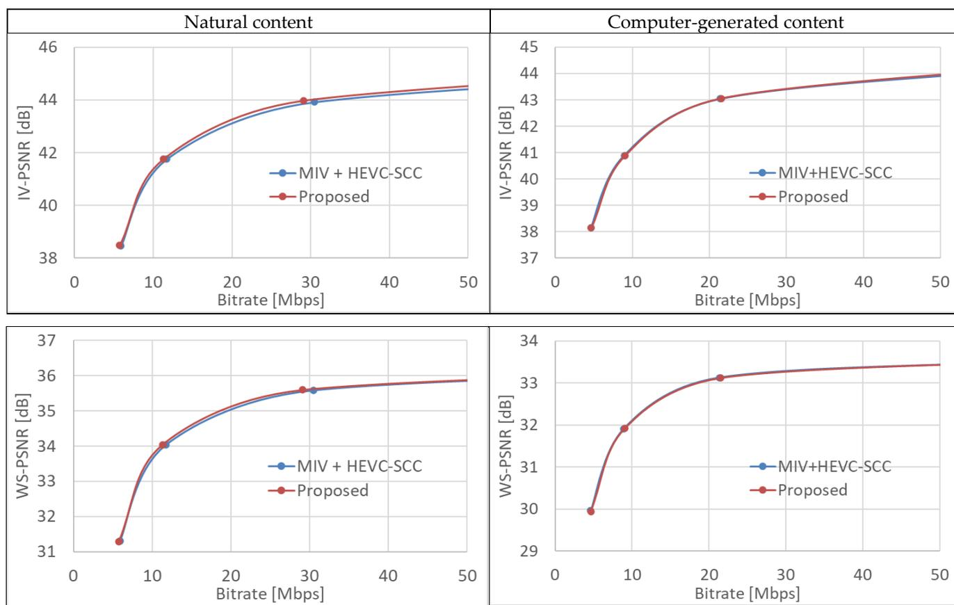
**Figure 4.** IV-PSNR and WS-PSNR RD-curves for natural content (**left**) and computer-generated content (**right**); comparison of basic HEVC-SCC and proposed SCC with quarter-pel IBC accuracy and tile-based IBC analysis for first texture atlas.
