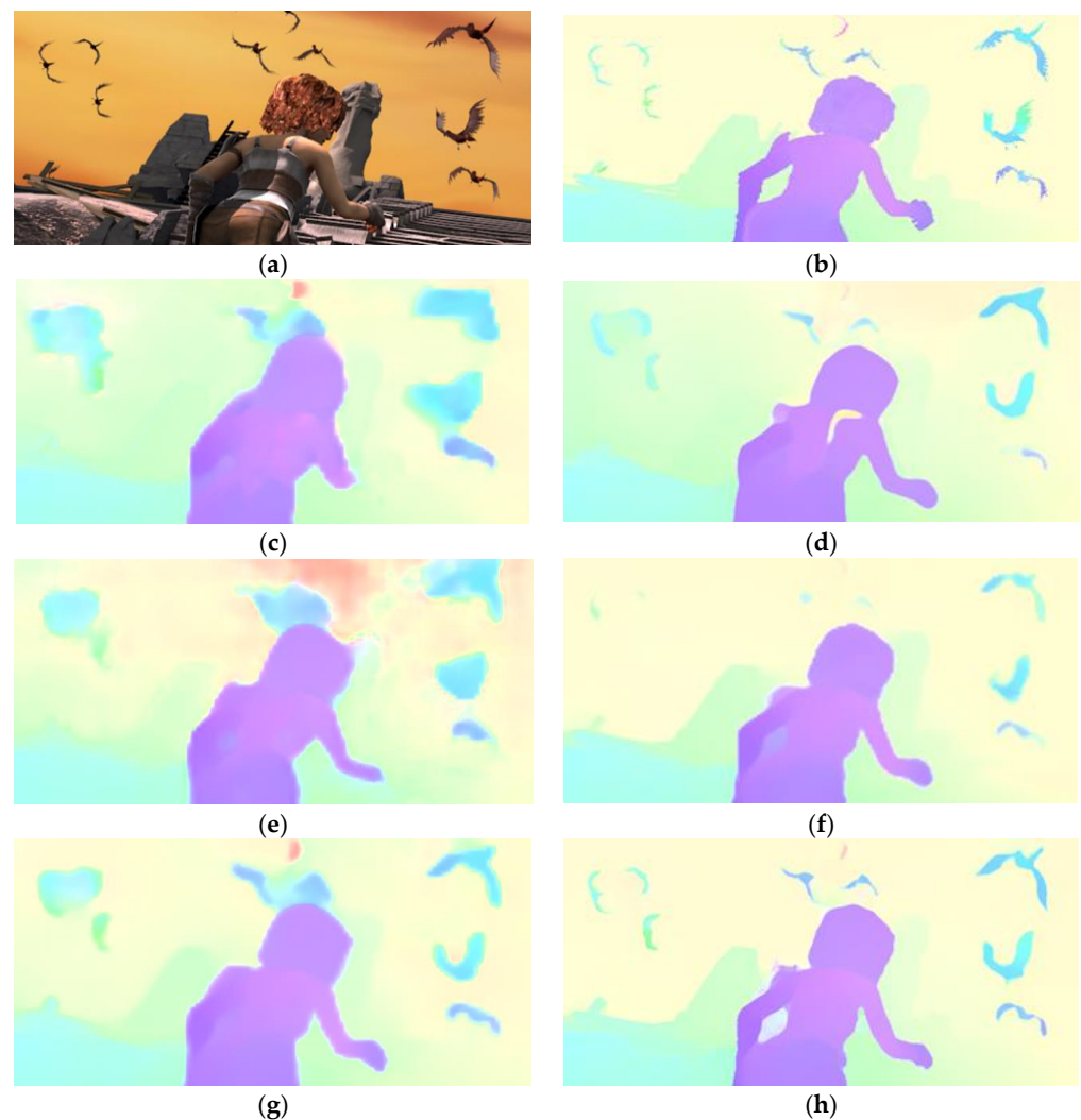
Figure 18. Visual comparison of optical flow fields estimated by different motion estimators: (a) Temple1; (b) ground truth; (c) ARFlow [25]; (d) FlowNet2 [22]; (e) PWC-Net [23]; (f) MaskFlowNet [47]; (g) LiteFlowNet3 [48]; (h) DCN-Flow.
