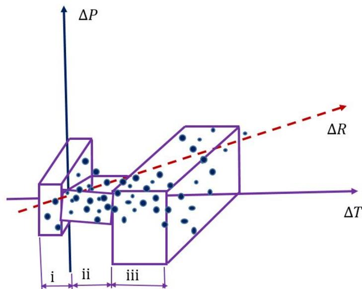
**Figure 3.** Flexibility requirement by a set of net load deviations over three regulation intervals: (i) primary, (ii) secondary, and (iii) tertiary.
