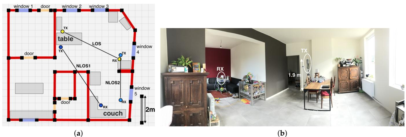
**Figure 3.** Living room environment. (a) Floor plan; (b) Picture of non-Line-of-Sight (NLOS) measurement setup NLOS2 with obstructed path distance 4.7 m.
