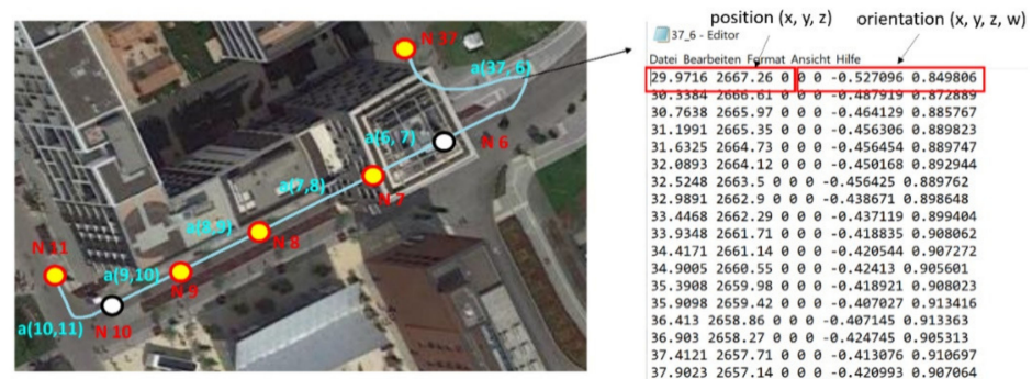
Figure 12. Path between nodes with ID 37 and 11 and recorded states of the vehicle associated with the graph edge between nodes with ID 37 and 6.
