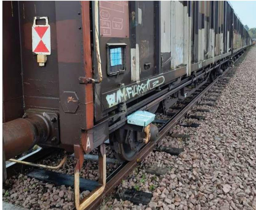
**Figure 19.** Placement of the nodes in the wagon.
