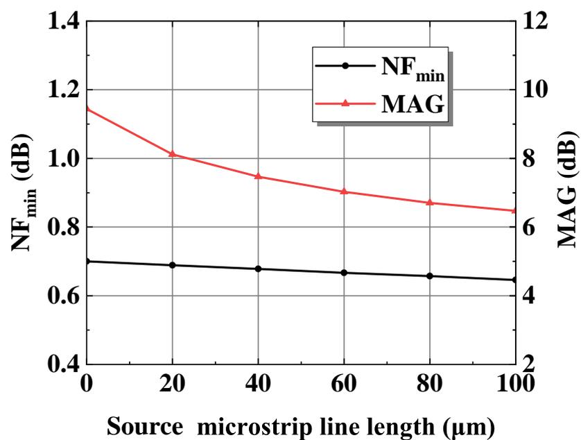
Figure 5. Simulated  $NF_{min}$  and MAG versus various values of source microstrip line length.
