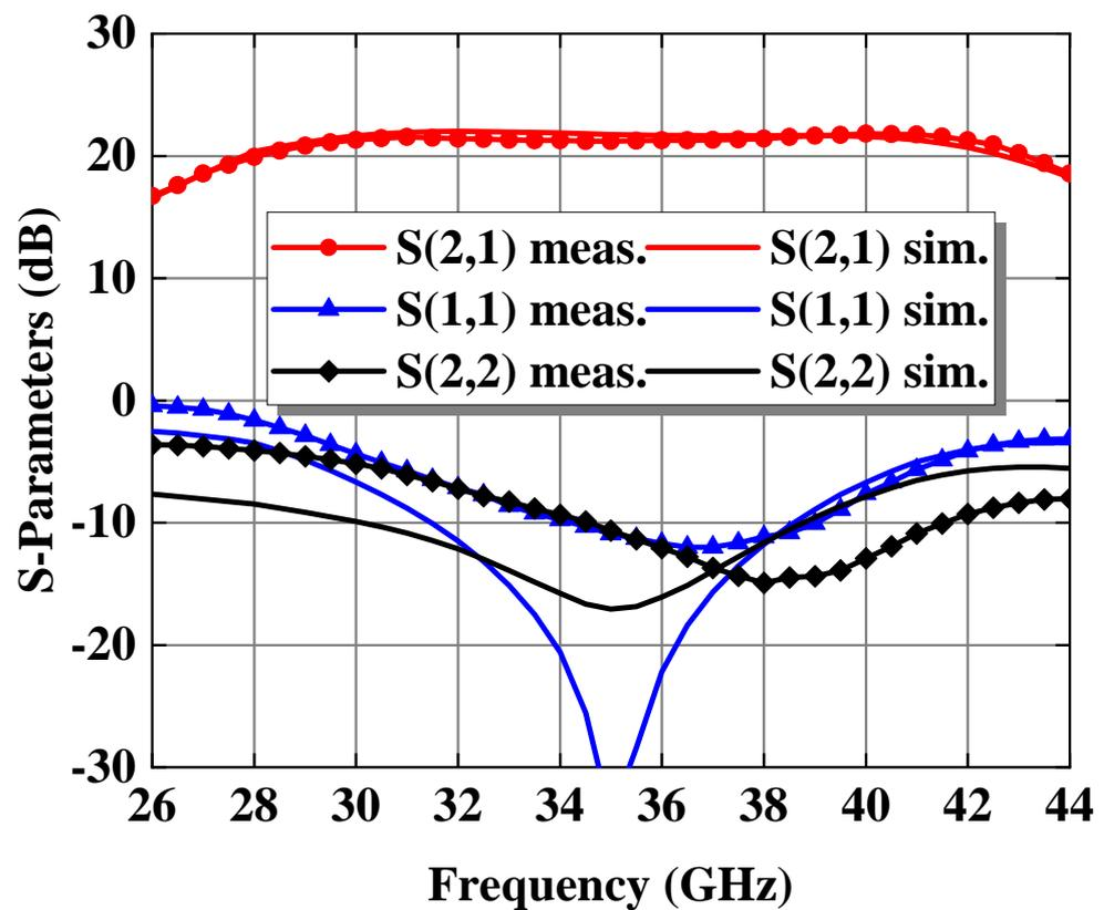
Figure 12. Simulated and measured S-parameters of the design.
