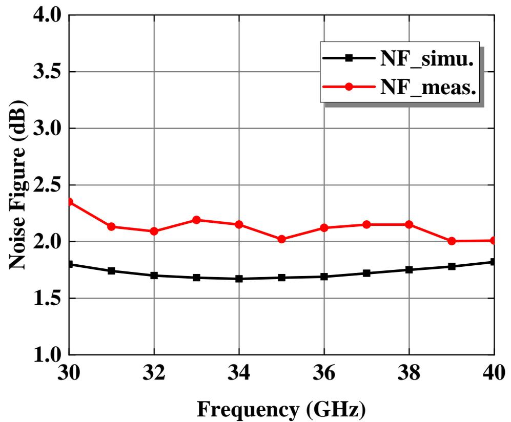
Figure 13. Simulated and measured noise figure.
