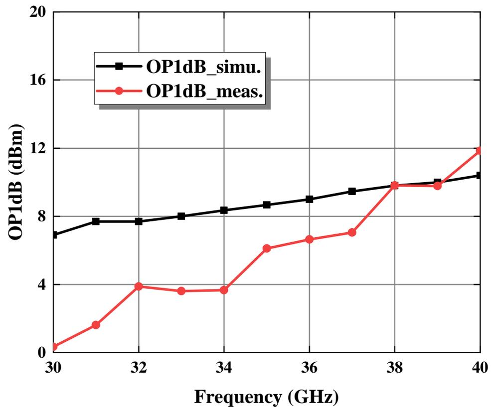
Figure 14. Simulated and measured output 1 dB compression point.
