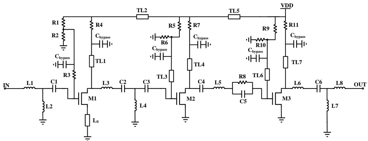
Figure 1. Schematic view of the proposed LNA.
