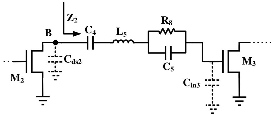
Figure 8. Small-signal equivalent model of the second stage.
