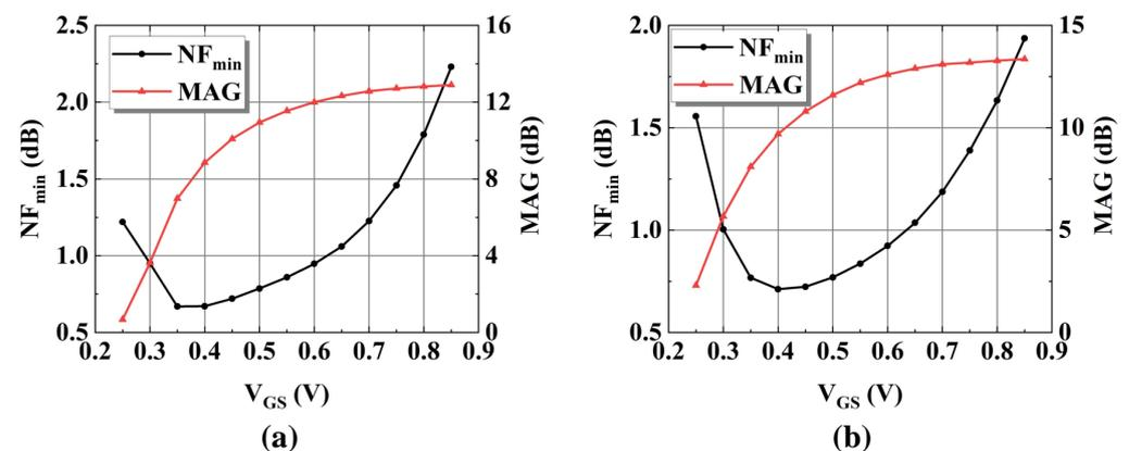
**Figure 2.** Simulated  $NF_{min}$  and MAG of a  $4 \times 25 \mu\text{m}$  (a) CPW; (b) MS transistor versus different values of  $V_{GS}$ .
