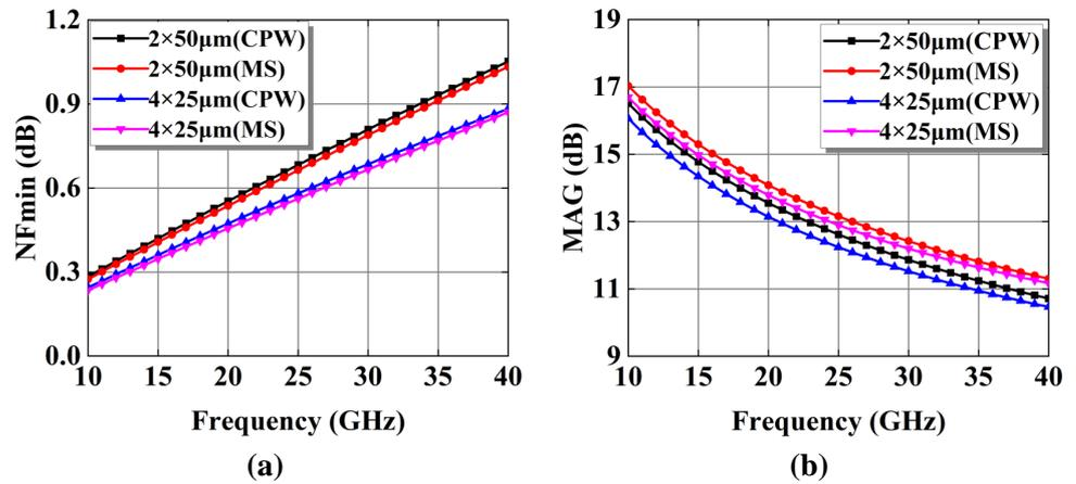
**Figure 3.** The simulated (a)  $NF_{min}$ ; (b) MAG for transistor of different sizes ( $2 \times 50 \mu\text{m}$  CPW,  $2 \times 50 \mu\text{m}$  MS,  $4 \times 25 \mu\text{m}$  CPW,  $4 \times 25 \mu\text{m}$  MS).
