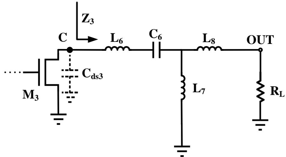
Figure 10. Small-signal equivalent model of the third stage.
