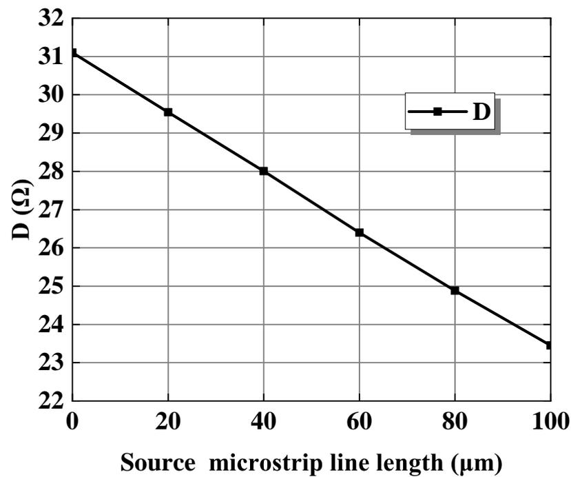
Figure 4. Simulated D versus different values of the source microstrip line length.
