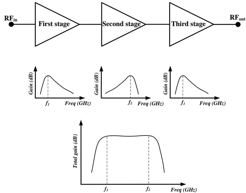
Figure 6. Block diagram of the stagger tuning technique.
