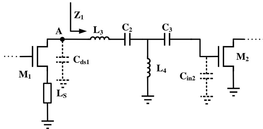
Figure 7. Small-signal equivalent model of the first stage.
