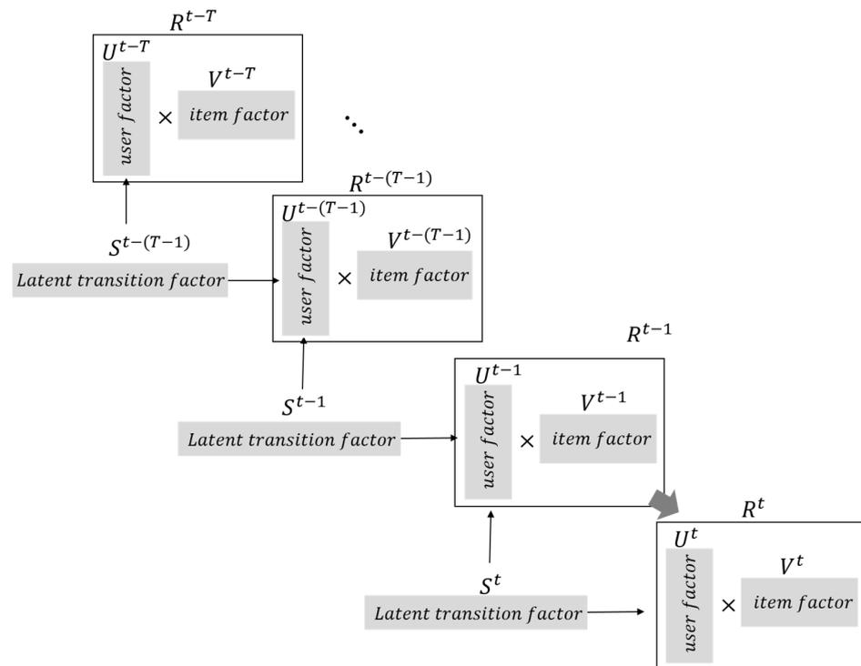
Figure 3. MF process with preference transition matrices.
