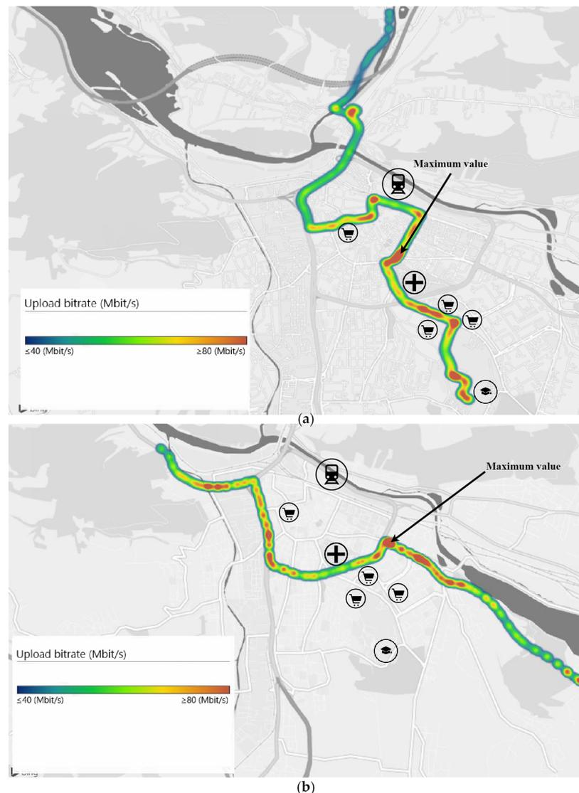
**Figure 5.** Average uplink speed on the route (a) number 1 and (b) number 2.
