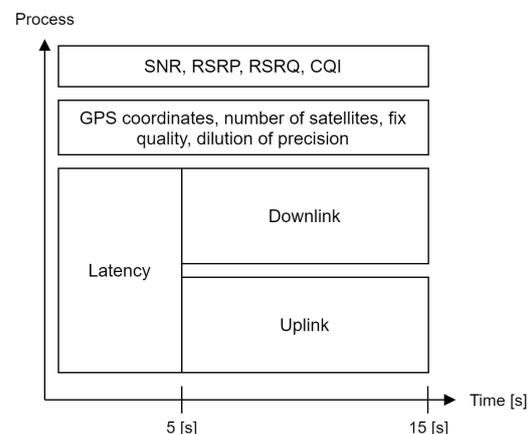
**Figure 2.** Proposed process for 5G communication and localization parameters research.
