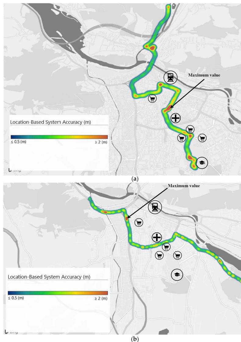
**Figure 7.** Average localization accuracy on route (a) number 1 and (b) number 2.
