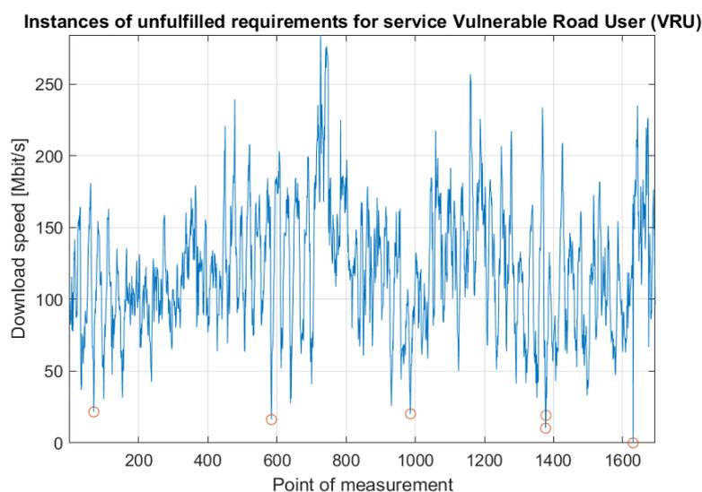
**Figure 9.** Visual representation of points in which downlink speeds do not meet the requirements of a service Vulnerable Road User (VRU).
