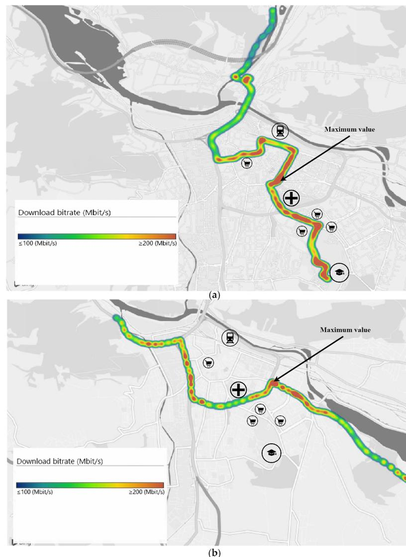
**Figure 4.** Average downlink speed on the route (a) number 1 and (b) number 2.
