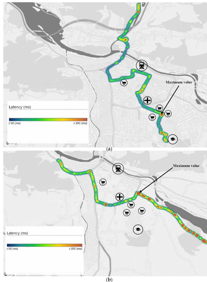
**Figure 6.** Average communication latency on the route (a) number 1 (b) and number 2.
