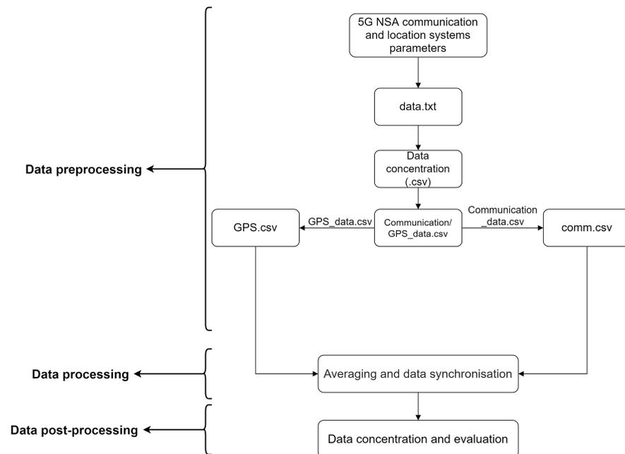
**Figure 3.** Proposed data processing of 5G communication and localization parameters.
