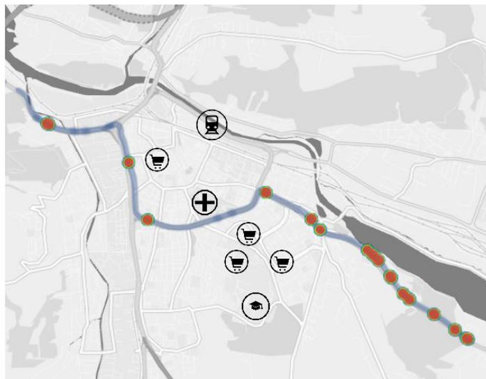
**Figure 13.** Identification of underserved sections in terms of uplink on Route 2.
