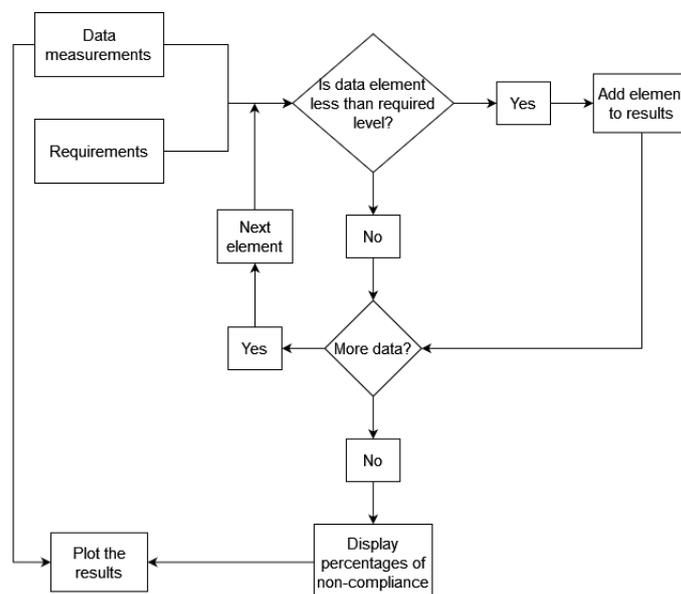
Figure 8. Non-Compliance Calculation and Visualization Flowchart.
