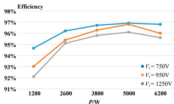
Figure 18. Efficiency curves of SDBuck-LLC under different input voltages  $V_i$ .
