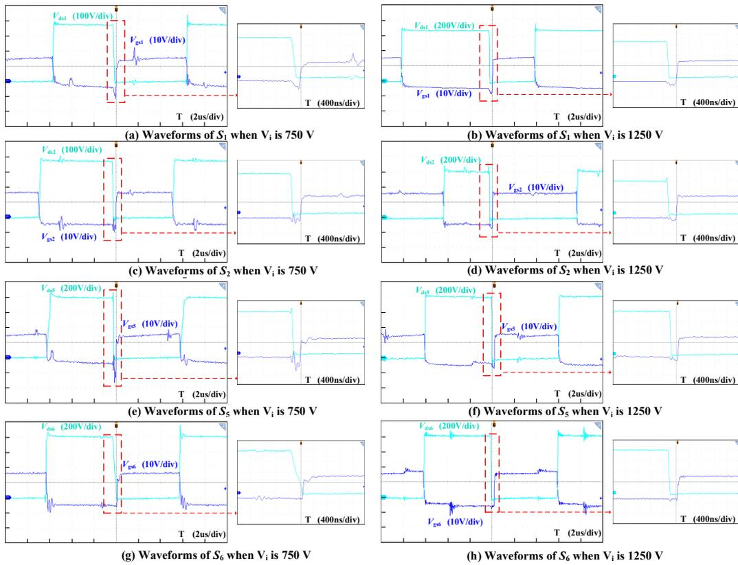
Figure 16. ZVS waveforms of each switch under full load and different input voltages  $V_i$ .
