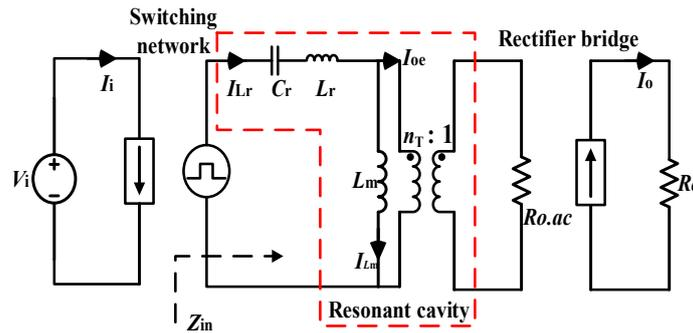
Figure 8. Steady-state equivalent circuit of SDBuck-LLC.
