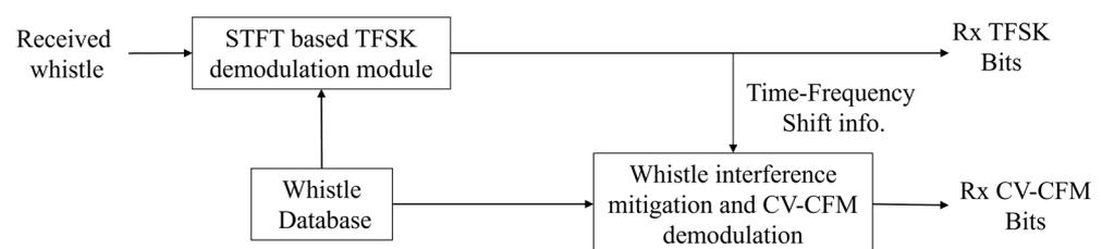
Figure 5. The block diagram of the proposed demodulation method.
