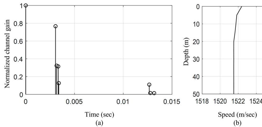
Figure 8. The simulation channel (a) delay profile, (b) SSP.
