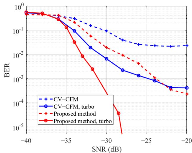
Figure 9. The UWA Channel simulation BER results.
