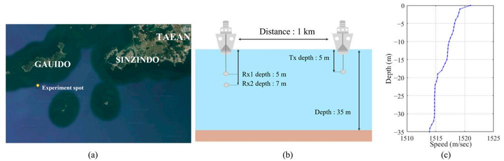
**Figure 10.** Ocean experiments environments (a) Location, (b) Configurations, (c) SSP.
