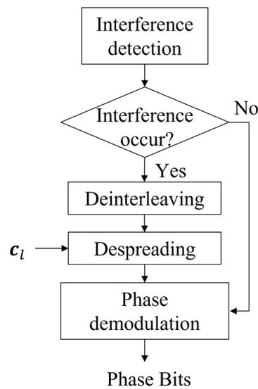
Figure 6. Despreading phase demodulation method.
