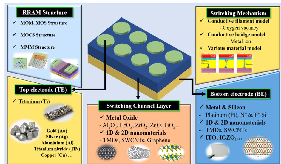
**Figure 1.** Illustration of structures, switching mechanisms, and various materials for RRAM device applications.
