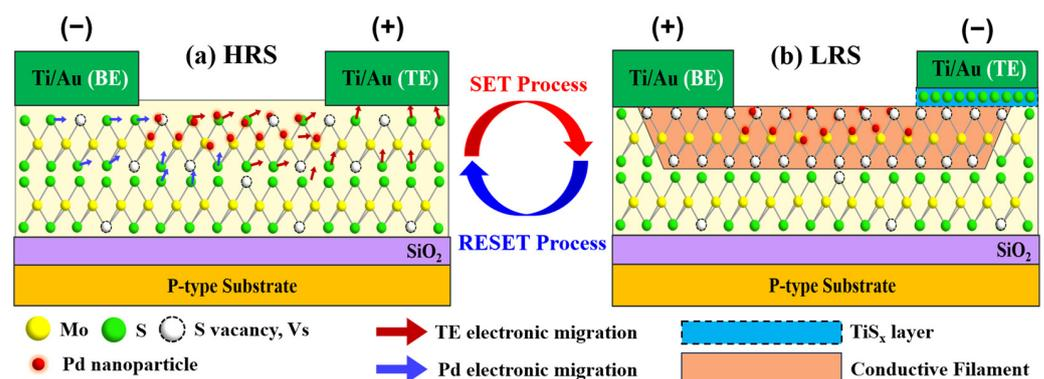
**Figure 5.** Resistive switching (RS) behavior in the Pd nanoparticle coating multilayer MoS<sub>2</sub> RRAM device is depicted. A schematic representation of the mechanisms for the lateral conductive filaments (CFs)-based RRAM device is shown: (a) High-resistance state (HRS, initial state); (b) Low-resistance state (LRS, after the SET process). The red and blue arrows indicate the direction of S-ion migration (electronic migration by TE and electronic migration by Pd).
