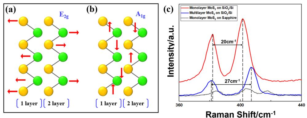
**Figure 3.** (a) E<sub>2g</sub> band in-plane vibration of MoS<sub>2</sub>; (b) A<sub>1g</sub> band out-of-plane vibration of MoS<sub>2</sub>; (c) Raman spectrum of monolayer MoS<sub>2</sub> and multilayer MoS<sub>2</sub> on the SiO<sub>2</sub>/Si. Two vibrational modes (E<sub>2g</sub> and A<sub>1g</sub>) of MoS<sub>2</sub>.
