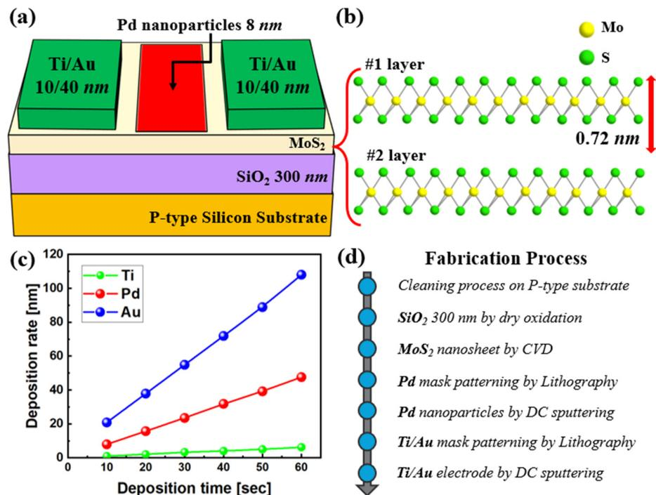
**Figure 2.** (a) The schematic diagram of the lateral-CF-based RRAM device with the Pd nanoparticles/MoS<sub>2</sub> nanosheet switching layer between the Ti/Au top electrode and Ti/Au bottom electrode; (b) The structure of monolayer MoS<sub>2</sub> (0.72 nm) or multilayer MoS<sub>2</sub> (1.44 nm) lattice layer; (c) Deposition rates of various metals (Ti, Pd, and Au) via DC sputtering; (d) The process flow chart illustrating the fabrication of the proposed RRAM architecture.
