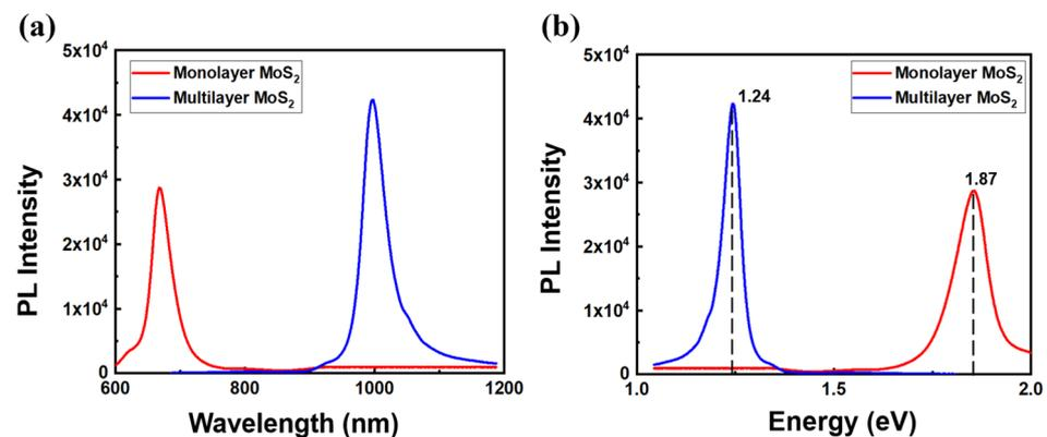
**Figure 4.** The scanning PL spectrum of both monolayer MoS<sub>2</sub> and multilayer MoS<sub>2</sub>; (a) Wavelength; (b) Energy bandgap of the emitted photon.
