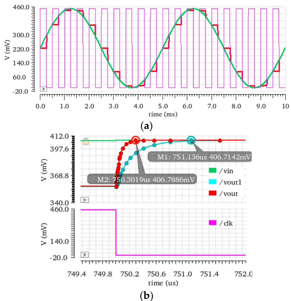
**Figure 3.** (a) Transient response of novel bootstrap switch. (b) Transient response with low  $V_t$  and standard  $V_t$ .
