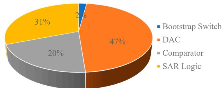
**Figure 11.** Power breakdown.
