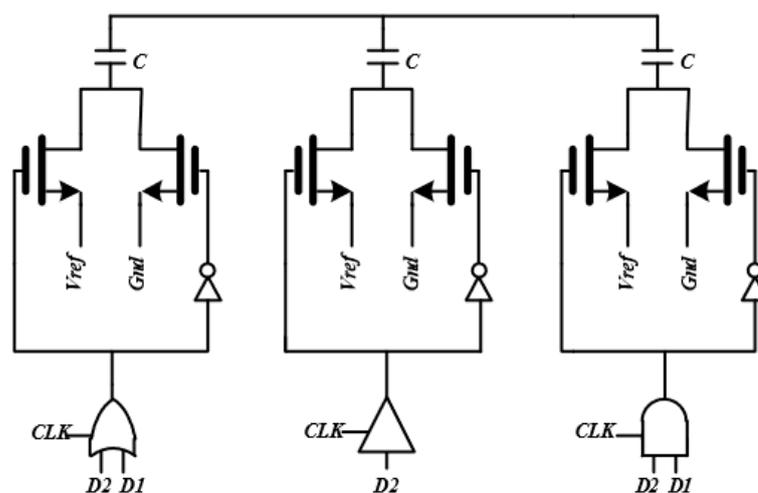
**Figure 7.** DAC capacitors along with 2-bit binary to thermometer decoding [13].
