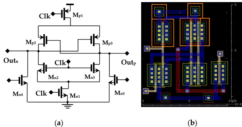
Figure 5. (a) Proposed dynamic comparator and (b) its layout.
