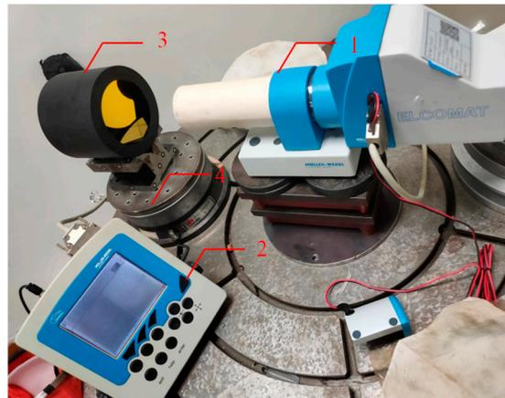
**Figure 3.** Angle measuring system based on the hollow corner cube prism. (1—photoelectric autocollimator, 2—display, 3—hollow corner cube prism, 4—precise angle dividing table).
