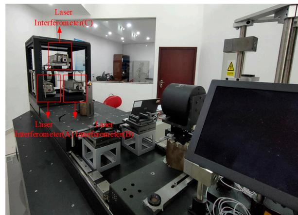
**Figure 1.** Laser interferometer system (standard value data acquisition).
