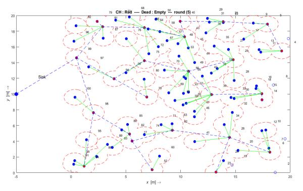
Figure 4. LSTM experiment in MATLAB (Red-cluster head, Blue-child node).
