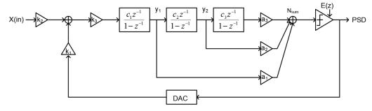
Figure 3. Proposed single-loop third-order modulator topology.
