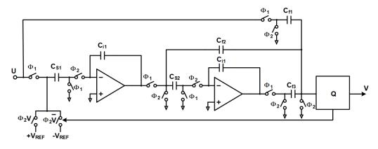
Figure 2. Schematic of the feedforward topology.
