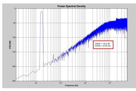
Figure 4. Ideal output spectrum with a 16 Hz input signal.
