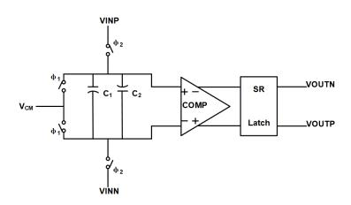
Figure 8. Schematic of the single-bit quantizer.
