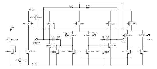
Figure 7. Schematic of the OTA in the modulator.
