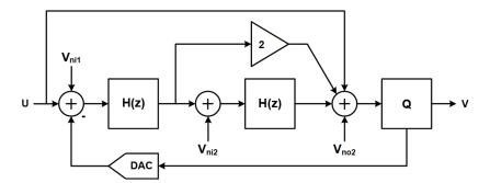
Figure 1. Noise sources in the feedforward topology.
