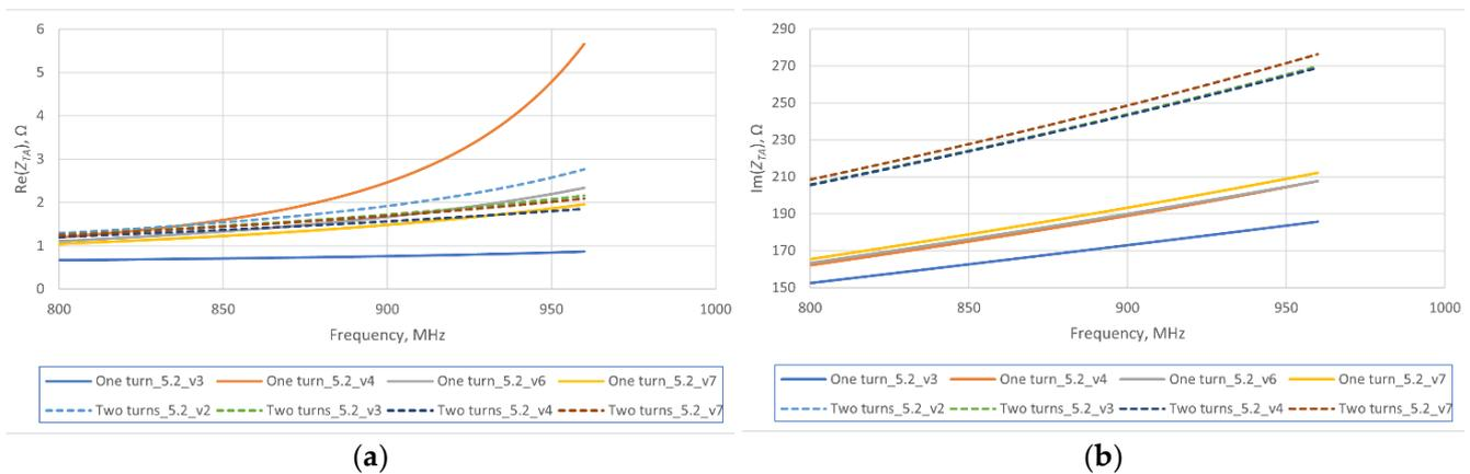
**Figure 6.** Antenna impedance  $Z_{TA}$  calculations for microelectronic module with 5.2 mm diameter: (a) real part of  $Z_{TA}$ ; (b) imaginary part of  $Z_{TA}$ .
