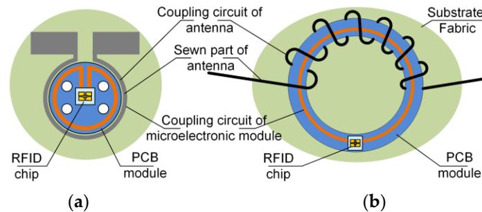
**Figure 3.** RFIDtex transponder: (a) primary solution of coupling system; (b) coupling system according to new conception of threaded bead.
