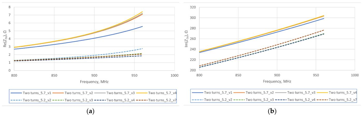
**Figure 7.** Antenna impedance  $Z_{TA}$  calculations for microelectronic module with 5.2 mm and 5.7 mm diameter: (a) real part of  $Z_{TA}$ ; (b) imaginary part of  $Z_{TA}$ .
