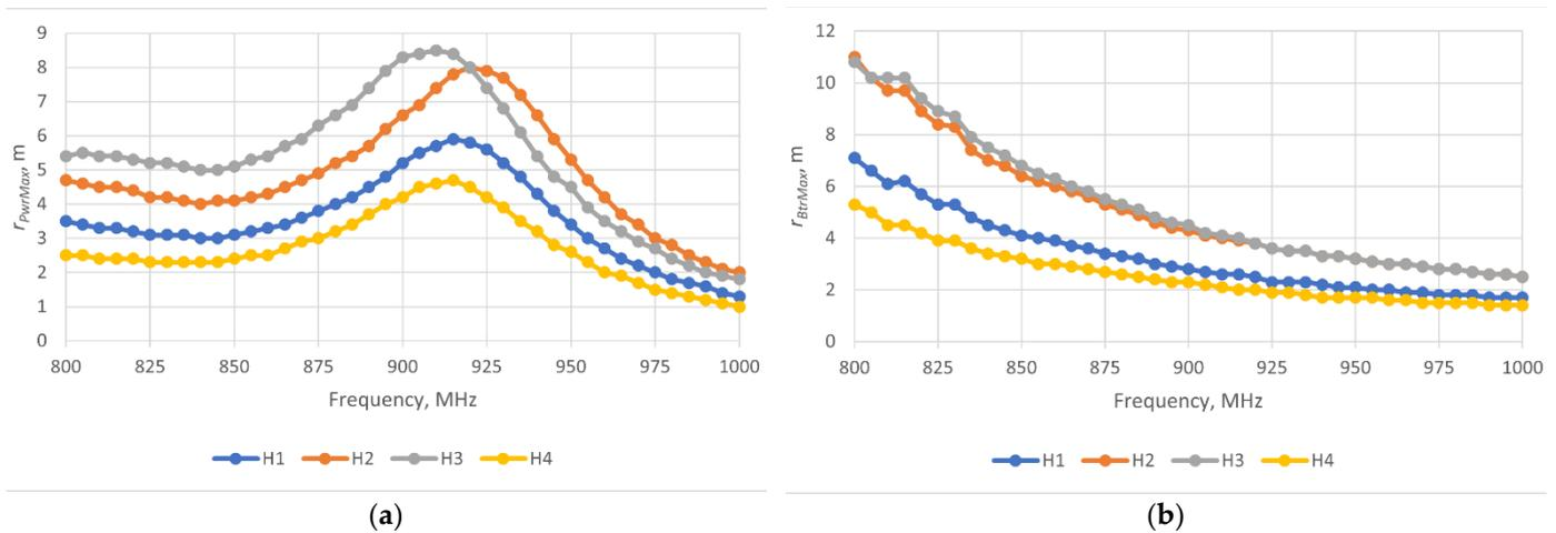
**Figure 11.** Theoretical read range: (a) in forward  $r_{PwrMax}$  and (b) reverse  $r_{BtrMax}$  direction.
