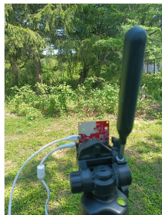
Figure 7. The experiment setup with AWR1642 BOOST mmWave radar, mounted on tripod.
