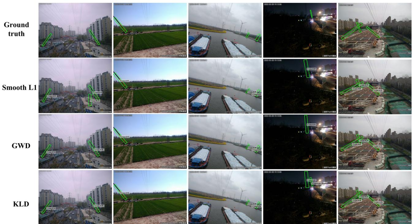
**Figure 6.** Experimental results of YOLOv8-Crane using various rotating object losses.
