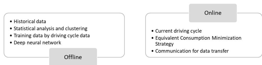
Figure 13. Overview of offline and online method for EV clustering proposed in [72].
