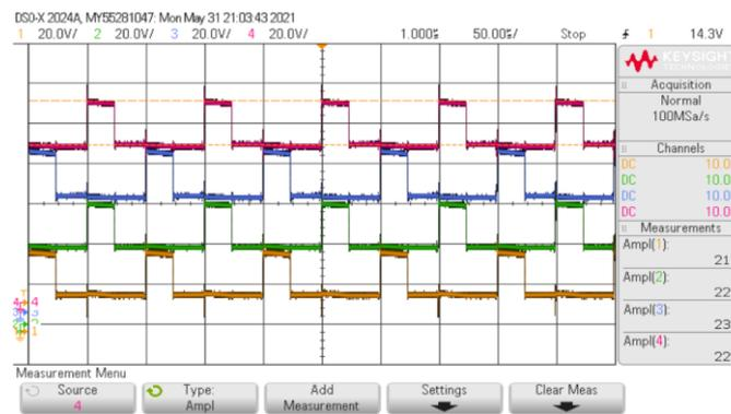
Figure 19. Node voltages  $V_1$  to  $V_4$  of SCC in buck mode.
