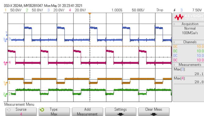
Figure 18. Drain-source voltages of  $S_1$  and  $S_2$  in buck mode.
