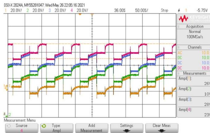
Figure 15. Node voltage  $V_5$  to  $V_8$  of the SCC in boost mode.
