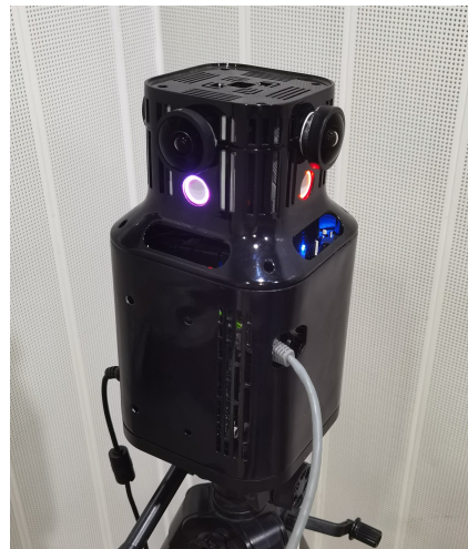
Figure 9. Four fisheye camera, integrated with projection transformation, compression coding, and network transmission modules.
