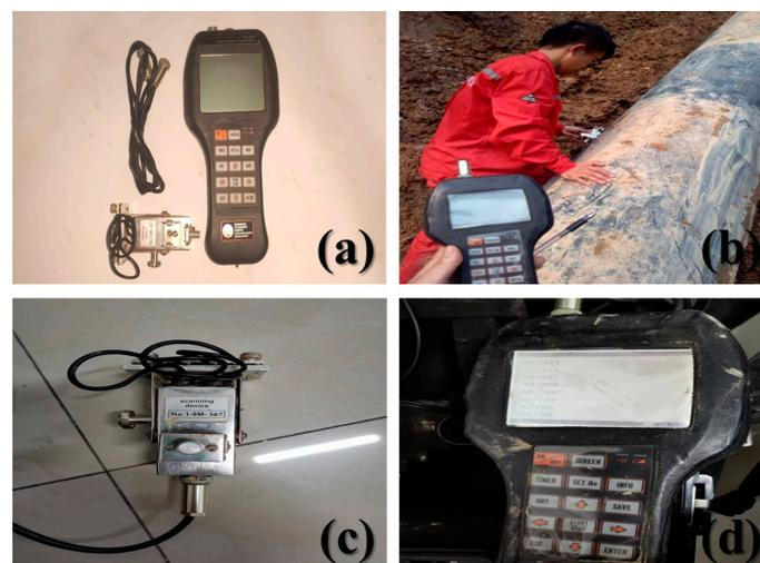
**Figure 2.** Non-contact 3D magnetic testing system. (a) The whole testing instrument; (b) Field operation; (c) data collector; (d) data analyzer.
