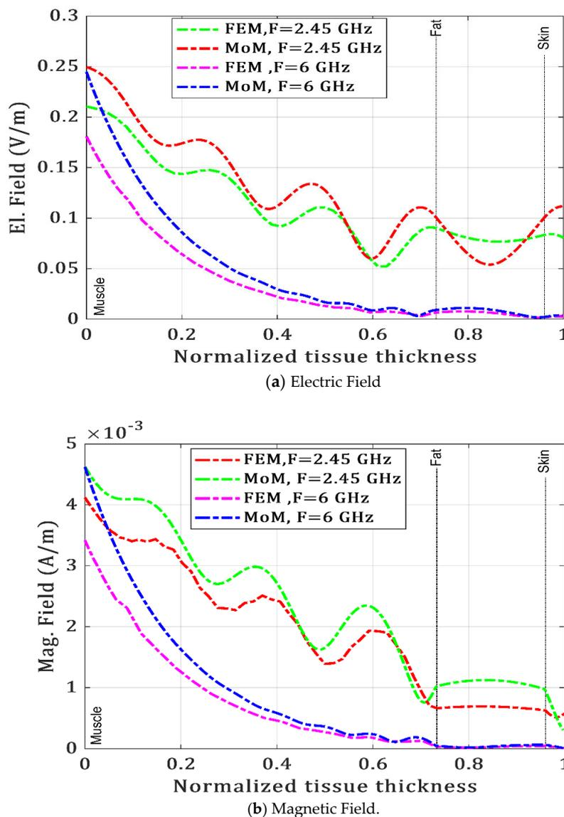
Figure 8. The EM field obtained by the MoM and FEM for IB2OB communication.
