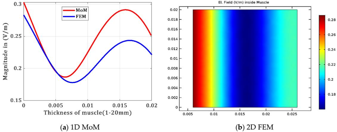
Figure 4. E-field inside muscle tissue for both methods at 915 MHz.
