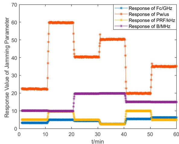
Figure 8. Dynamic response curve of the jamming parameter matrix over time.
