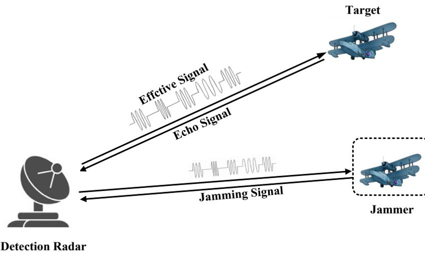
Figure 1. Electronic jamming system.
