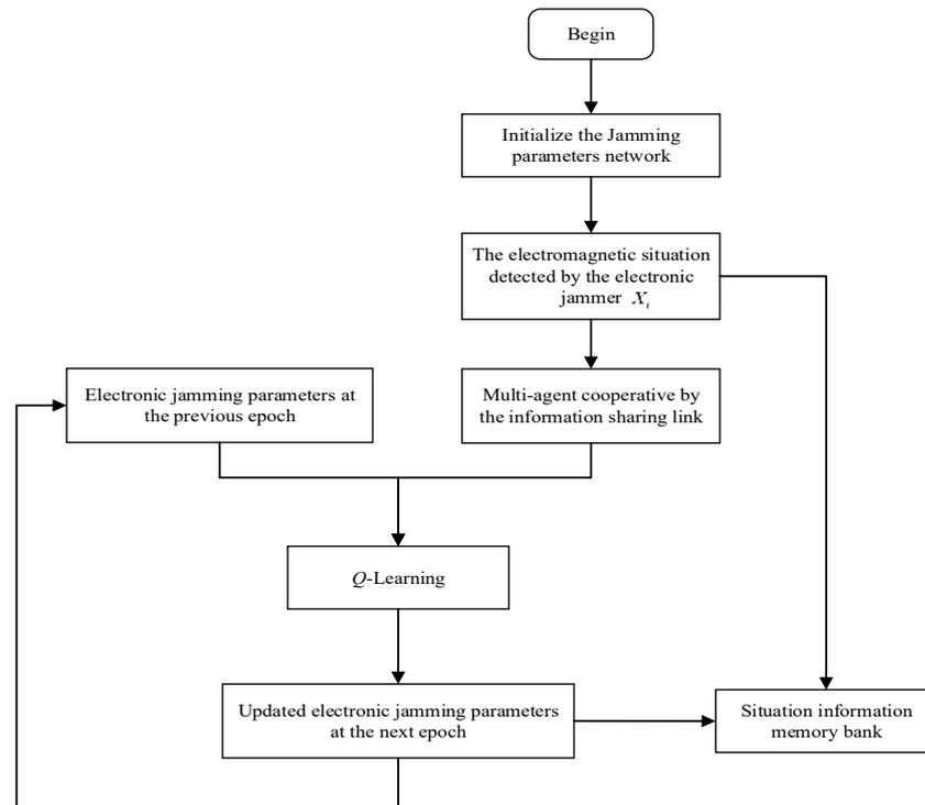
Figure 4. Electronic jamming flow chart based on multi-agent information sharing and Q-learning methods.
