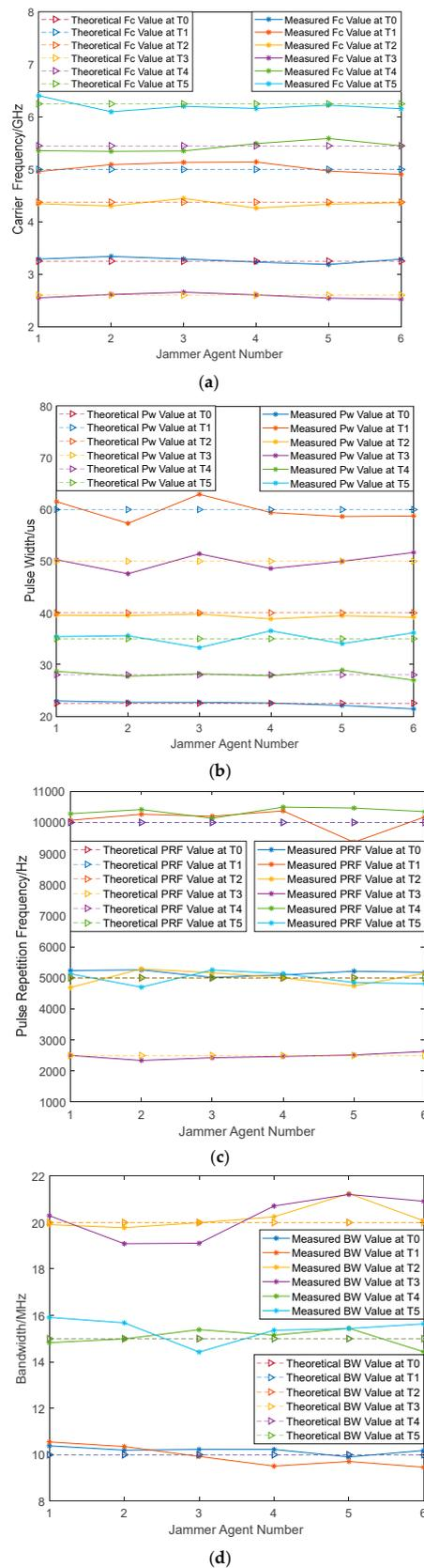
**Figure 5.** The multi-agent electronic jammer measures the electromagnetic situation information at different times. (a) The measurements and theoretical values of  $F_c$ ; (b) the measurements and theoretical values of  $PW$ ; (c) the measurements and theoretical values of  $PRF$ ; (d) the measurements and theoretical values of  $BW$ .
