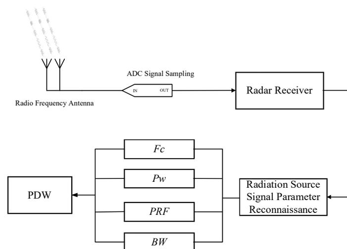
Figure 3. The estimation process of electromagnetic parameters of radiation sources.
