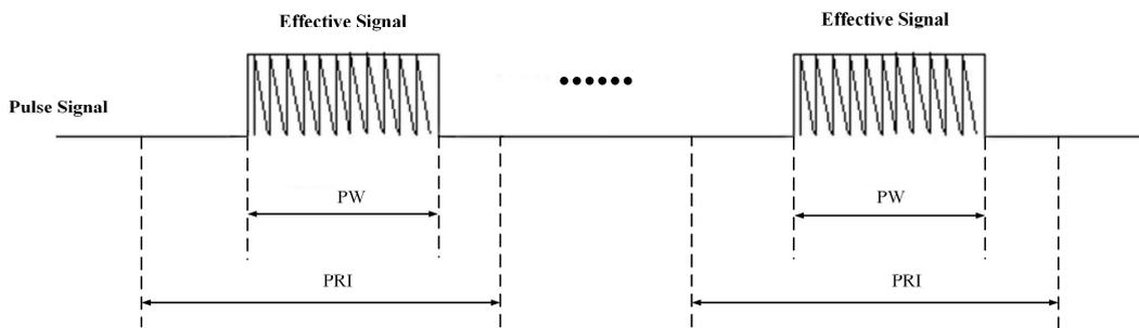
Figure 2. Pulse energy detection and pulse width measurement.
