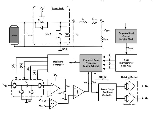
**Figure 2.** Proposed twin frequency control DC-DC buck converter using accurate load current sensing technique.
