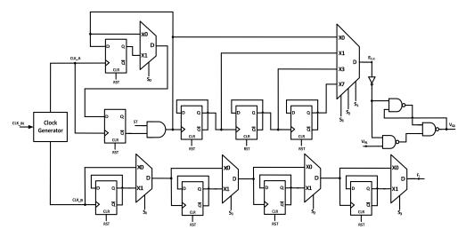
Figure 5. Proposed twin frequency control scheme (TFCS).
