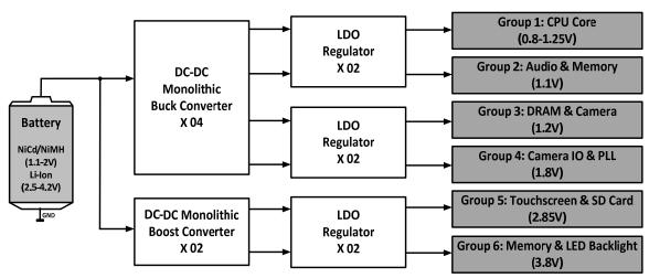
**Figure 1.** A vital part of the 3G/4G smartphone power management unit (PMU).
