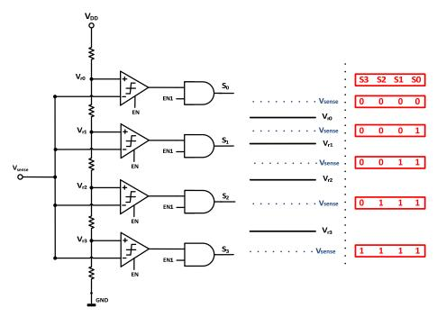
Figure 4. Four-bit thermometer code ADC.
