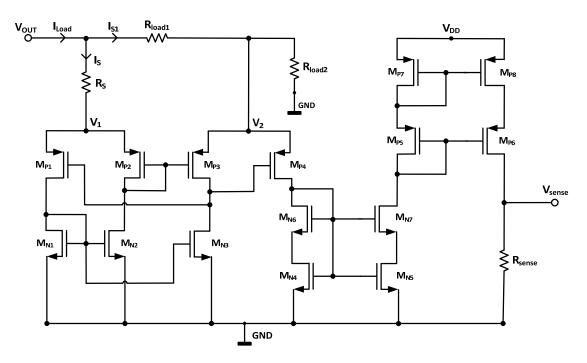
Figure 3. Accurate load current sensing (ALCS) block.
