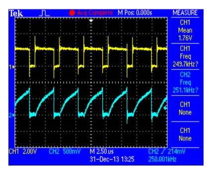
**Figure 9.** Peak efficiency achieved—waveform of  $V_x$  and  $V_{\text{int}}$  ( $V_{BATT} = 2$  V,  $V_{out} = 1.25$  V, Freq = 250 kHz and  $I_{load} = 30$  mA).
