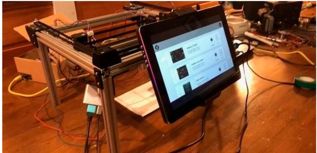
**Figure 3.** Original inspectAR implementation using a motorized XY frame and external touch display.
