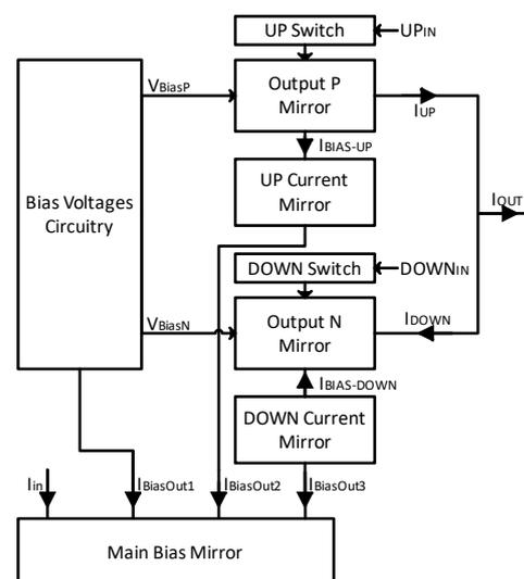
**Figure 1.** Block diagram of the CP. The arrows indicate the direction of the current flow for currents ( $I_{in}$ ,  $I_{BIASOut1}$ ,  $I_{BIASOut2}$ ,  $I_{BIASOut3}$ ,  $I_{BIAS-DOWN}$ ,  $I_{BIAS-UP}$ ,  $I_{DOWN}$ , and  $I_{UP}$ ) and the input/output direction for voltages ( $V_{BiasN}$ ,  $V_{BiasP}$ ,  $UP_{IN}$ , and  $DOWN_{IN}$ ).
