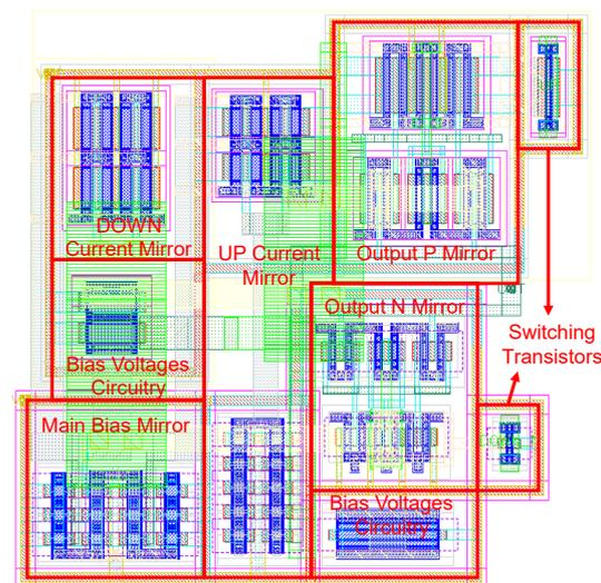
**Figure 3.** Layout of the proposed charge pump.
