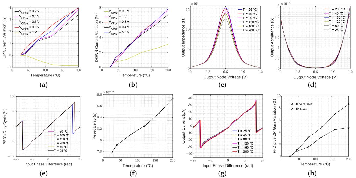
**Figure 12.** PFD and CP thermal characterization: percentage DC DOWN current variation in (a); percentage DC UP current variation in (b); CP’s output impedance in (c); CP’s output admittance in (d); PFD characteristic in (e); propagation delay of the PFD’s reset pa path in (f); PFD plus CP cascade characteristic in (g); PFD plus CP cascade’s UP and DOWN gain percentage variation in (h).
