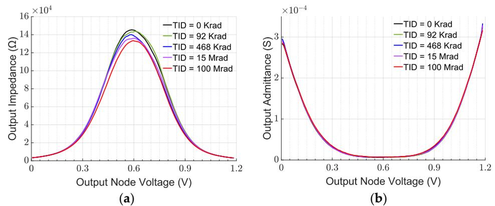
**Figure 13.** CP TID characterization: output impedance (a) and output admittance (b) for different TID levels.
