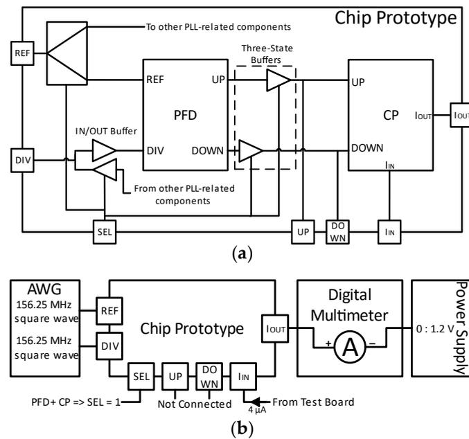
**Figure 7.** Block diagram of the PFD and CP in the chip prototype (a), and test setup for the PFD plus CP cascade (b).
