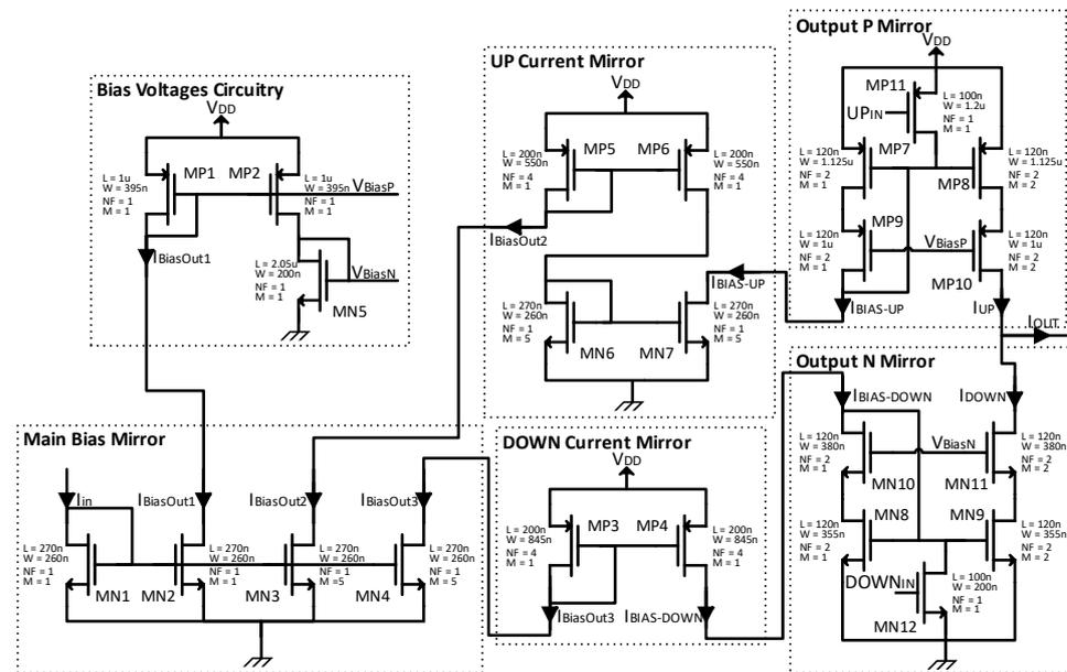
**Figure 2.** Detailed schematic of the CP.
