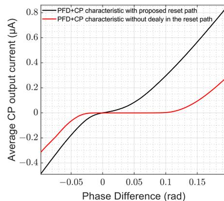
**Figure 5.** PFD-CP chain characteristic with proposed reset path design (black) and without delay in the reset path (red).
