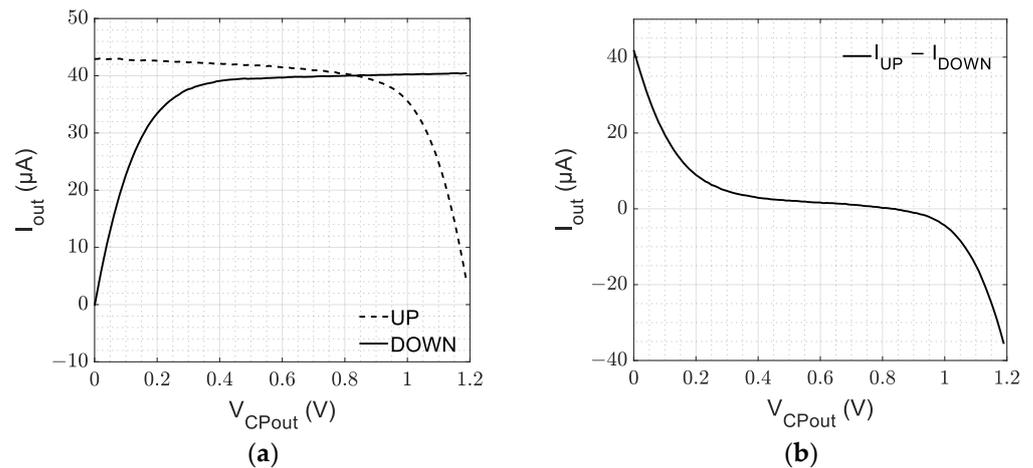
**Figure 8.** CP electrical DC characterization: (a) UP and DOWN currents; (b) total output current.
