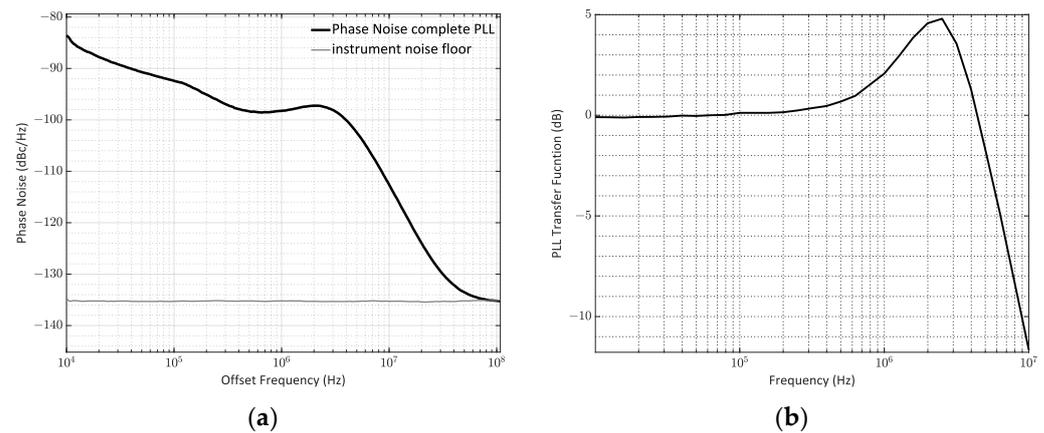
**Figure 11.** (a) Phase noise measurement of the complete PLL where the proposed CP and PFD were integrated. The measurement was carried out by exploiting a Rohde and Schwarz FSL18 Spectrum Analyzer (Rohde & Schwarz, Munich, Germany), whose noise floor is reported in the figure. (b) Phase transfer function of the complete PLL where the proposed CP and PFD were integrated. The measurements were performed by exploiting a MSO72304DX Tektronix Oscilloscope (Tektronix, Beaverton, OR, USA).
