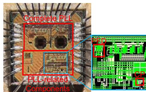
**Figure 6.** Chip prototype on the left; layout of the bottom-right corner of the chip prototype on the right.
