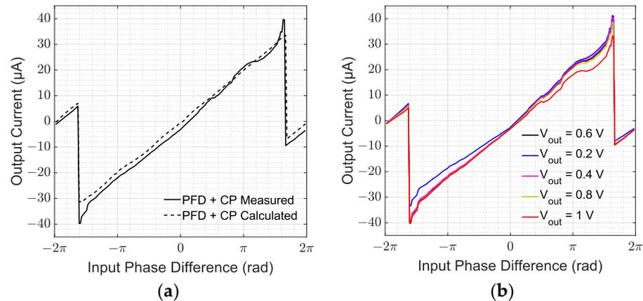
**Figure 10.** Measurement results of the cascaded PFD and CP: (a) measured characteristic with an output node voltage of 0.6 V vs. that calculated from the measures of the CP and PFD taken separately; (b) measured characteristic for different output node voltages.
