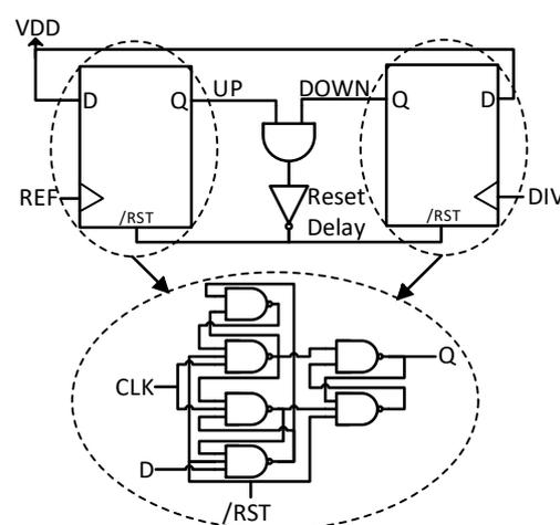
**Figure 4.** Block scheme of the PFD.
