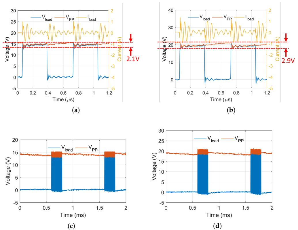
Figure 10. Waveforms on a microsecond scale of the voltage on the load  $V_{load}$ , the output voltage of the charge pump  $V_{PP}$ , and the current on the load  $I_{load}$  with a power supply of (a) 3.7 V and (b) 5 V. Waveforms on a millisecond scale of  $V_{load}$  and  $V_{PP}$  with a power supply of (c) 3.7 V and (d) 5 V.
