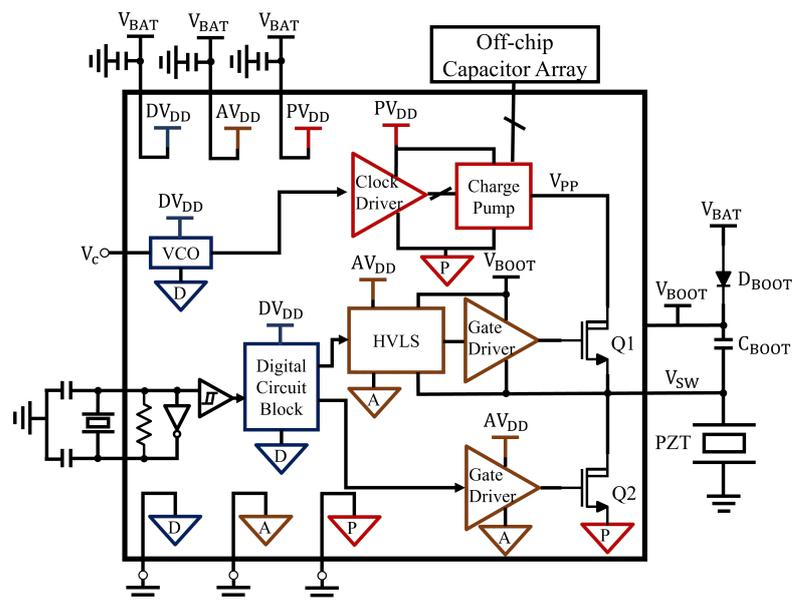
**Figure 2.** System architecture of the proposed ASIC and its periphery components. The blue boxes are digital modules, the brown boxes are analog modules, and the red boxes are power modules.
