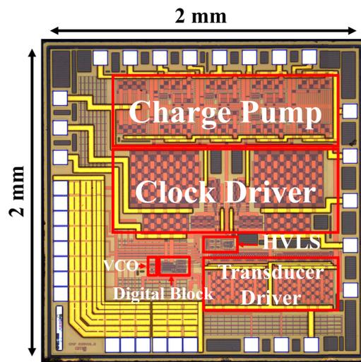
Figure 7. Micrograph of the bare die.
