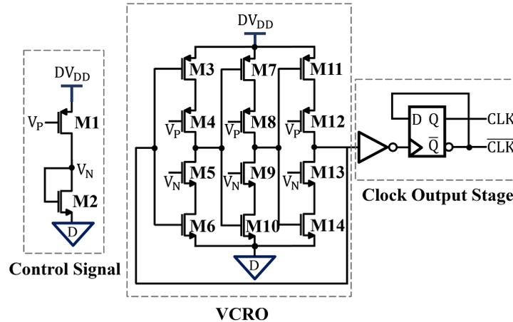
Figure 6. Circuit diagram of the 3-stage current-starved voltage-controlled oscillator.
