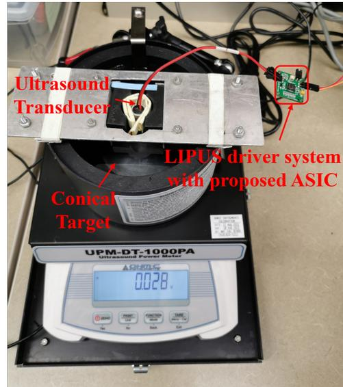
Figure 9. The ultrasound power measurement setup.
