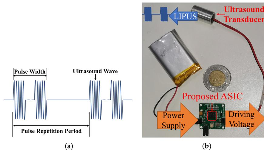
**Figure 1.** (a) Demonstration of a LIPUS wave. (b) The proposed highly integrated LIPUS system compared with a Canadian 2 CAD coin.
