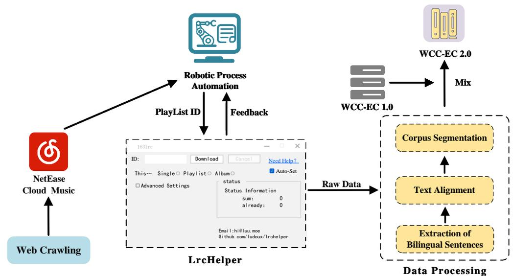
Figure 2. Process of crawling WCC-EC 2.0.
