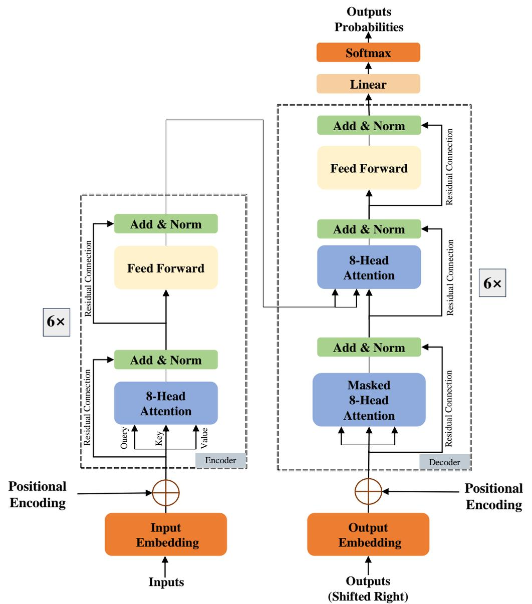
Figure 3. The architecture diagram of the transformers used in the experiment.
