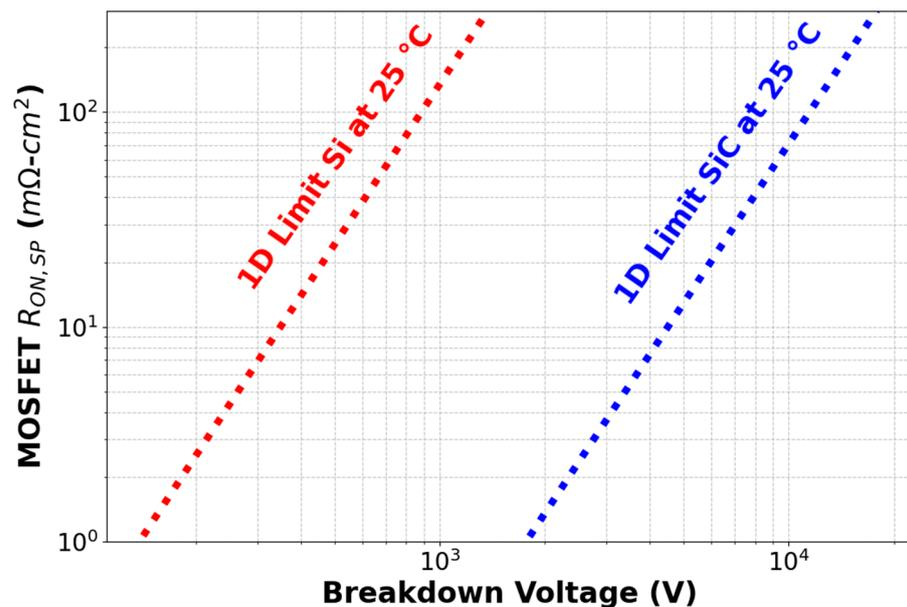
Figure 12. 1D specific on-resistance versus breakdown voltage comparing Si and SiC.
