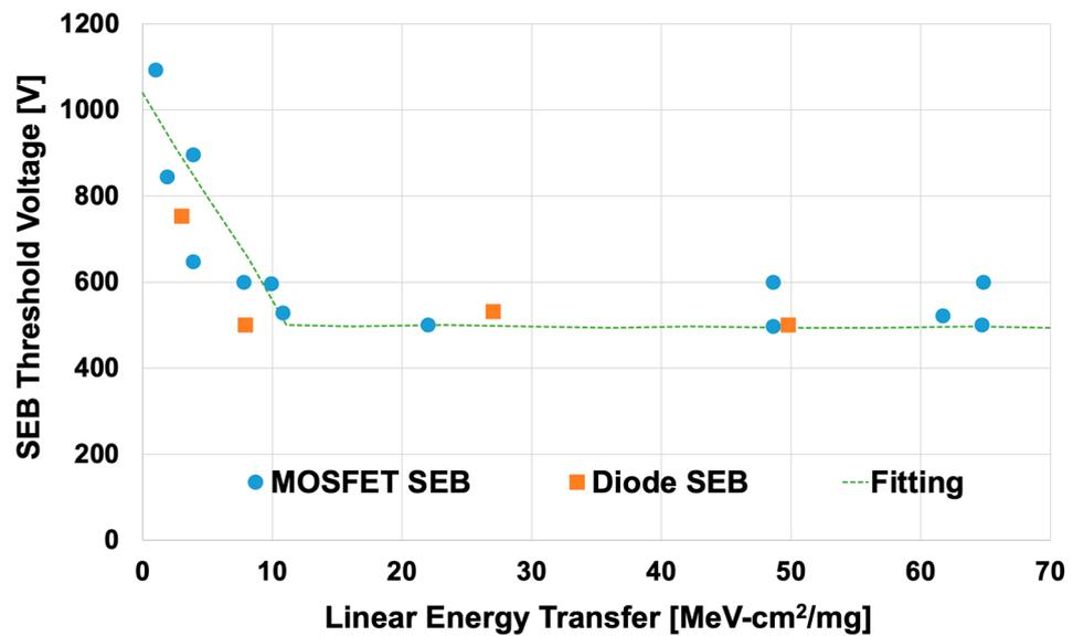
Figure 11. Experimentally determined SiC MOSFET and diode burnout threshold voltage, based on the data from [8,20].
