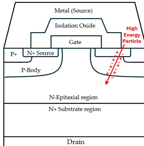
**Figure 2.** Traditional vertical power N-channel DMOSFET under high-energy particle strike at parasitic BJT region.
