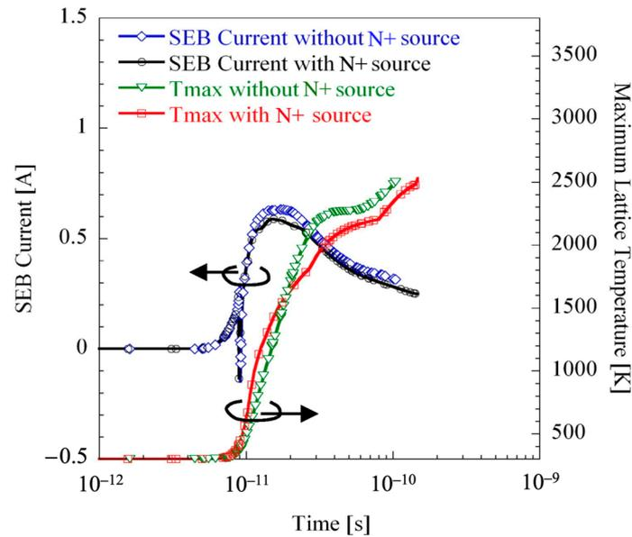
**Figure 7.** Simulated SEB currents and max lattice temperatures with and without the N+ source region in SiC MOSFET, reproduced from [22].
