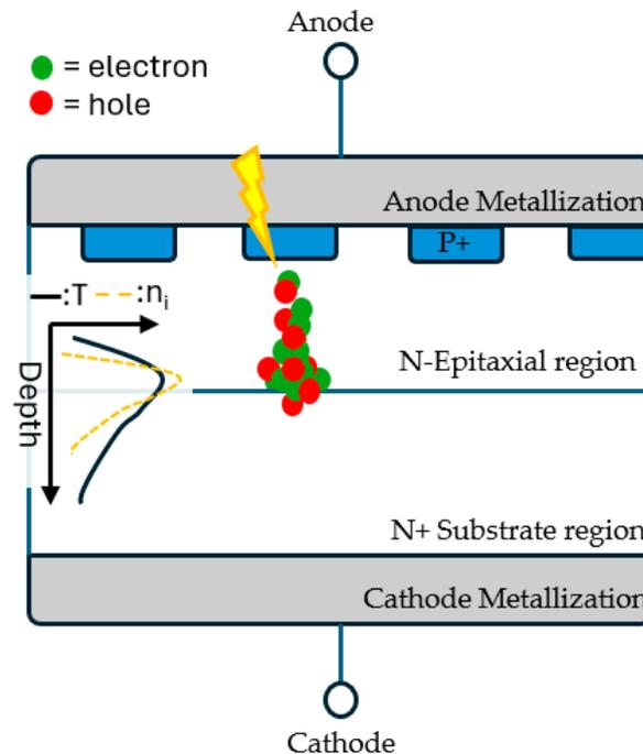
**Figure 3.** Power diode under radiation strike. Carriers generated from impact ionization with 1D intrinsic carrier concentration and device temperature response.
