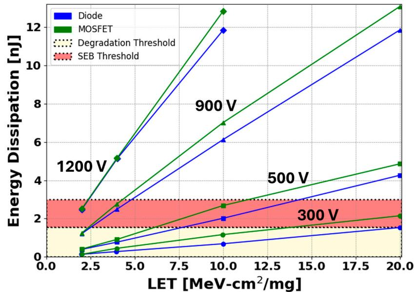
Figure 10. Calculated energy dissipation for 10 ps after heavy ion strike with degradation and SEB threshold conditions, based on the data from [20].
