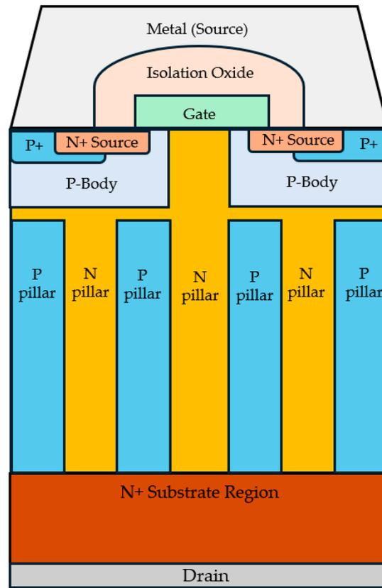
Figure 15. Traditional vertical N-channel double-diffused SJ MOSFET cross section (not to scale).
