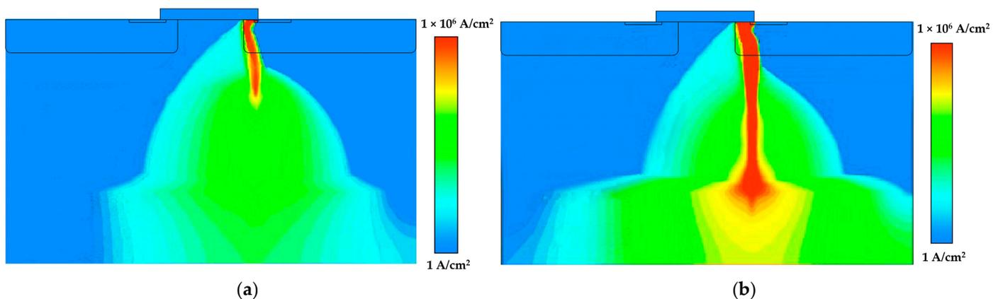
**Figure 6.** Electron current density contours of models with (a) impact ionization turned off, isolating for BJT contribution; (b) impact ionization turned on, based on the data from [8].
