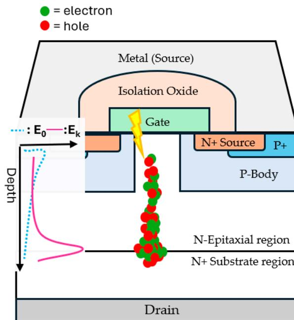
**Figure 8.** Vertical N-channel double-diffused power MOSFET under radiation strike with 1D electric field distribution and carrier mapping. The peak electric field shift or Kirk effect is illustrated.
