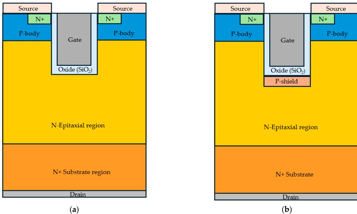
**Figure 13.** UMOSFET cross section (a) of a traditional vertical N-channel double-trench and (b) with a buried P-shield layer (not to scale).
