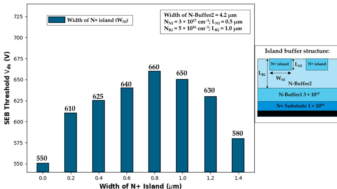
**Figure 14.** Island buffer layer SEB results and optimized design parameters, based on the data from [92].
