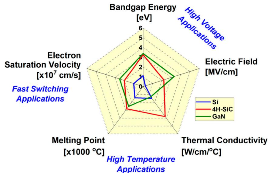
**Figure 1.** Material characteristic comparison between 4H-SiC, GaN, and Si, reproduced from [1].
