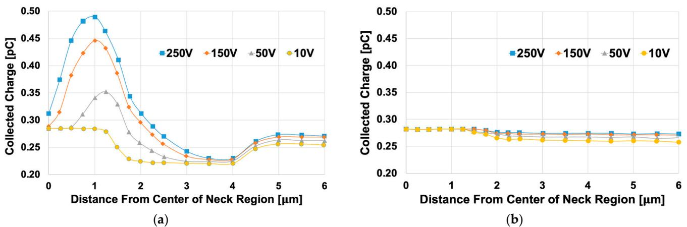
Figure 5. Collected charge simulation results of (a) MOSFETs; (b) diodes with respect to devices lateral position where ion strike occurs, based on the data from [25].
