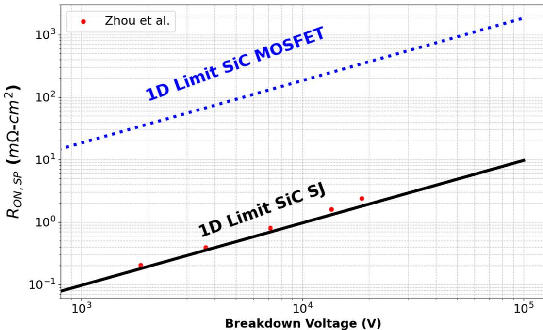
Figure 16. SiC 1D limit and SJ structure tradeoff with respect to Zhou et al. [109] vertical SJ model.
