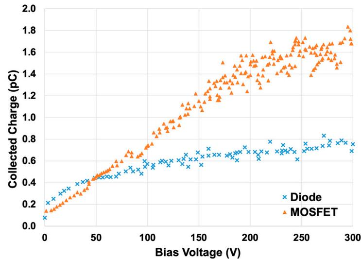
Figure 4. Diode and MOSFET collected charge at reverse biases of 0 to 300 V, based on the data from [25].
