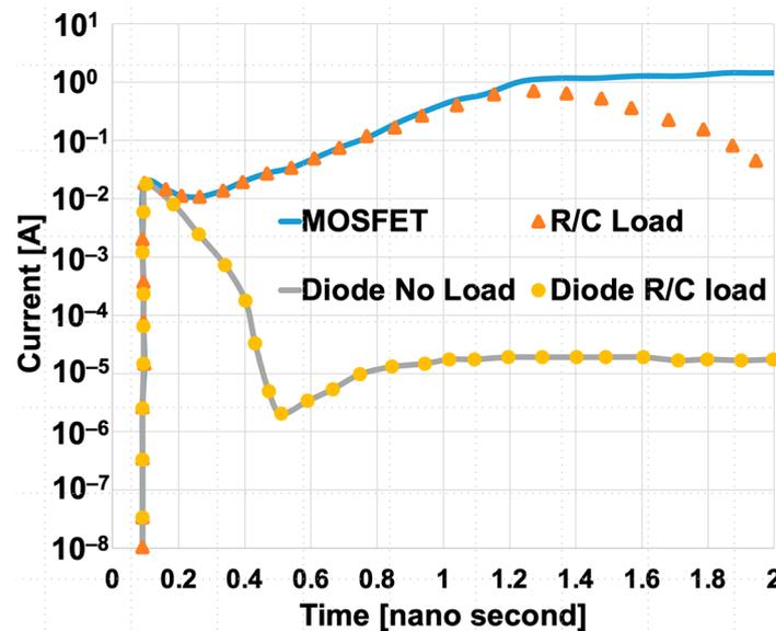
**Figure 9.** Current plot comparison of diode and MOSFET with and without implementation of the in-line resistor, based on the data from [20]. The diode matches the MOSFET for the first 0.15 ns, then responses begin to differ.
