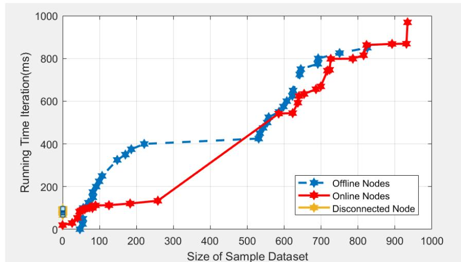
**Figure 6.** Running time for iteration on dataset by edge devices.
