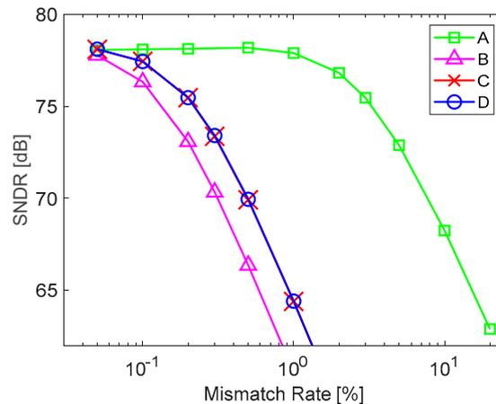
**Figure 6.** SNDR vs. Mismatch rate with and without DWA obtained from MATLAB behavioral simulations. Average of 100 iterations.  $N_{fft} = 2^{15}$ , and  $V_{IN} = -0.9$  dBFS. A and B, DWA not applied; C, DWA applied to 4-bit MSB and 4-bit LSB separately; D, DWA applied to 4-bit MSB only. A, mismatch is present in coarse CDAC only. B, C, and D, mismatch is present in fine CDAC only.
