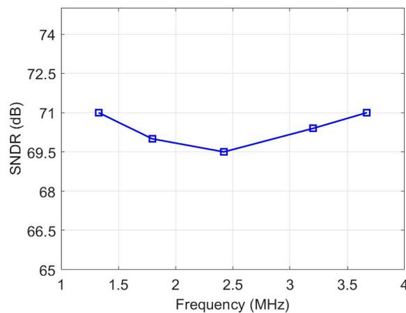
**Figure 15.** SNDR variation vs. input frequency obtained from Spectre transient noise simulations.
