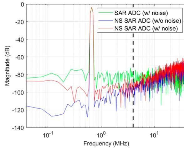
**Figure 13.** Output spectra obtained from Spectre transient simulations. Blue, NS-SAR ADC without noise; red, NS-SAR ADC with noise; green, SAR ADC with noise. Dashed line represents the signal bandwidth. ( $N_{fft} = 2048$ ,  $V_{IN} = -0.3$  dBFS,  $f_{sig} = 664$  kHz, Hann windowing.)
