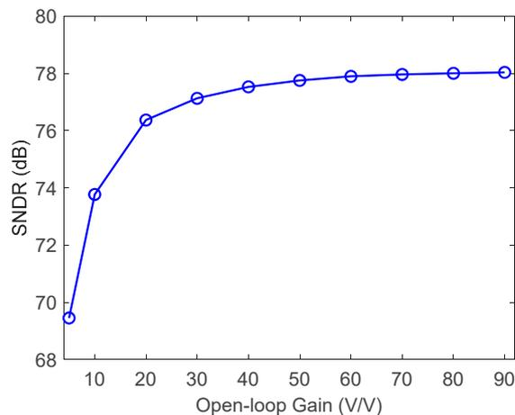
**Figure 5.** SNDR vs. open-loop gain from MATLAB behavioral simulations. ( $V_{IN} = -0.9$  dBFS).
