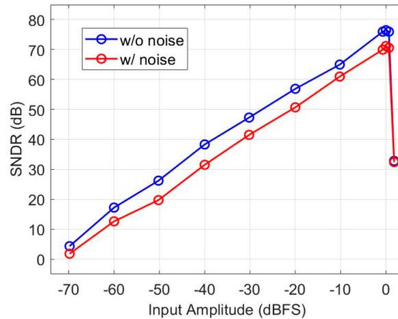
**Figure 14.** SNDR of the proposed ADC from Spectre transient simulations with and without noise.
