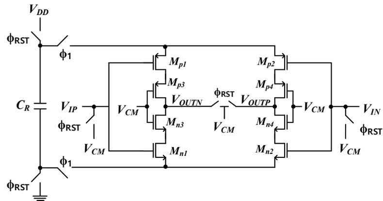
Figure 10. Schematic of the cascode FIA.
