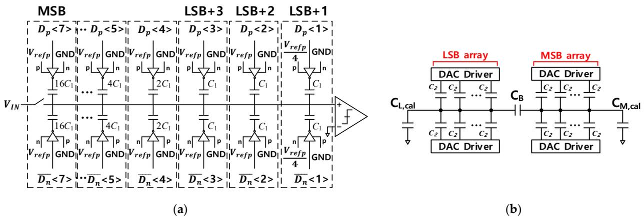
Figure 9. Schematic of the (a) coarse CDAC and (b) fine CDAC.
