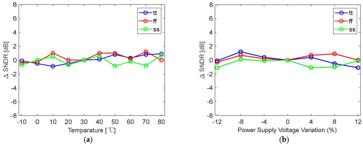
**Figure 16.** SNDR variation vs. (a) temperature and (b) power supply variations from Spectre transient noise simulations.
