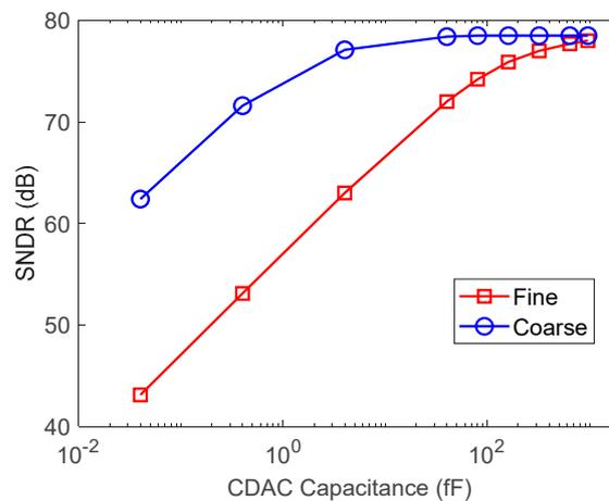
**Figure 8.** SNDR versus CDAC total capacitance.
