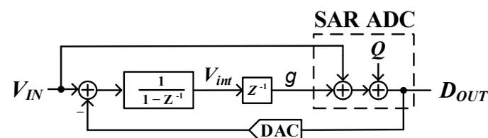
Figure 1. Signal flow diagram of the proposed NS-SAR ADC.
