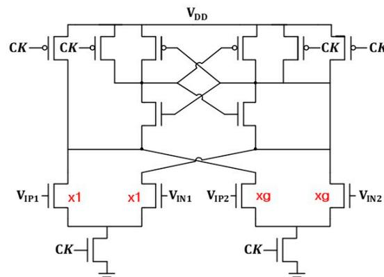
Figure 12. Schematic of the 2-input StrongArm latch comparator.
