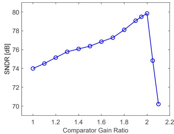
**Figure 4.** SNDR vs. normalized comparator gain ratio from MATLAB behavioral simulations. ( $A = 100$ ,  $V_{IN} = -0.9$  dBFS).
