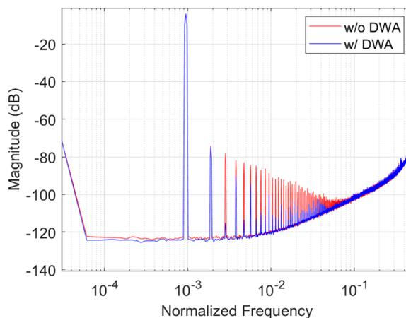
**Figure 7.** FFT spectra of the proposed NS-SAR ADC output with and without DWA obtained from MATLAB behavioral simulations. Average of 100 iterations.  $N_{fft} = 2^{15}$ ,  $\sigma_C = 0.5\%$ , and  $V_{IN} = -0.9$  dBFS.
