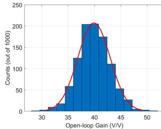
Figure 11. Simulated open-loop gain against process variations from Monte Carlo simulations (1000 runs).
