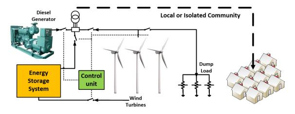
Figure 3. Schematic of the proposed hybrid system.
