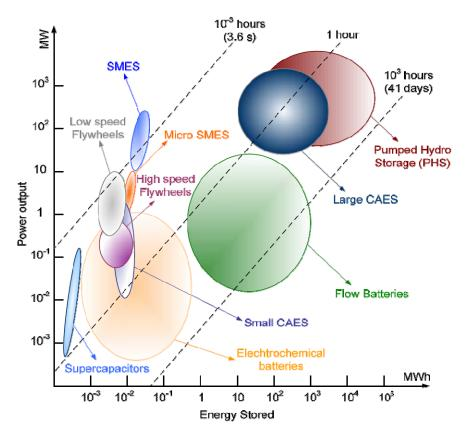
Figure 1. Energy storage systems with different storage capacity [9].
