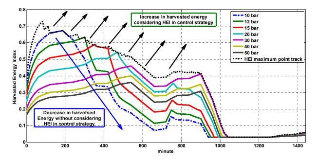
Figure 9. The calculated harvested energy index in different working pressures.
