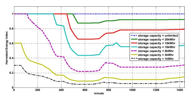
Figure 8. Harvested Energy index for different energy storage capacity.
