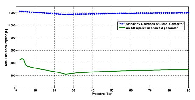
Figure 13. The DG fuel consumption in Standby and On-Off mode of operations.
