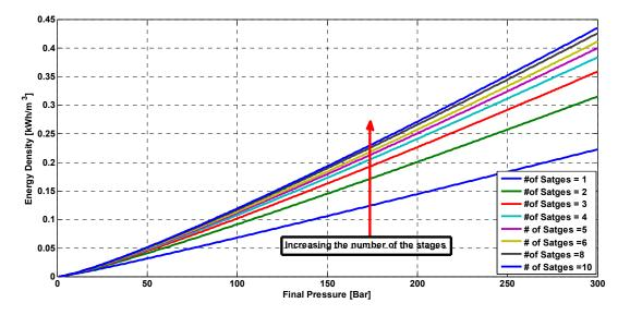
Figure 6. Energy density variation as function of number compression stages and pressure.
