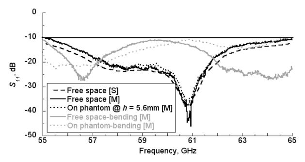
Figure 3. Bending antenna in *H*-plane on a semi-cylindrical skin-equivalent phantom with R = 15 mm.
