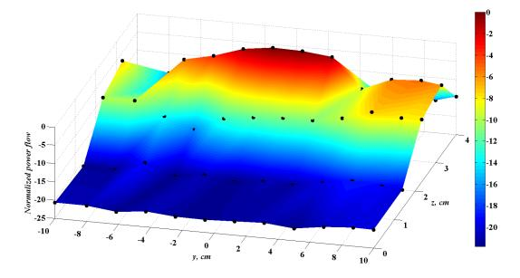
The data demonstrate that the path gain obtained with the rectangular phantom is similar to the one obtained with the realistic hand model (the maximum deviation is less than 6 dB). This suggests that this propagation path is robust and only slightly sensitive to the hand shape and posture. However, tilting the hand may strongly impact the path gain.
