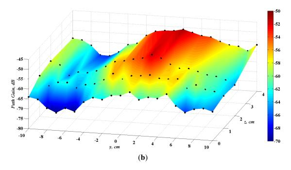
Figure 13. Computed normalized power flow distribution for rectangular skin-equivalent phantom at d = 5 cm.
