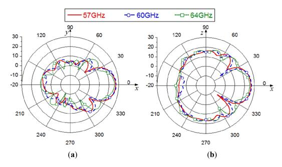
The measured radiation patterns in both *E* and *H* planes at 60 GHz of the antenna placed at a distance h = 5.6 mm on a flat skin-equivalent phantom are shown in Figure 6. As it can be seen, both *E*- and *H*-planes are strongly affected by the human body presence because of reflection from and absorption in the body.
