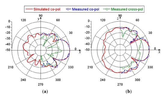
**Figure 4.** Measured and simulated radiation patterns in free space at 60 GHz: (a) *E*- and (b) *H*-planes.
