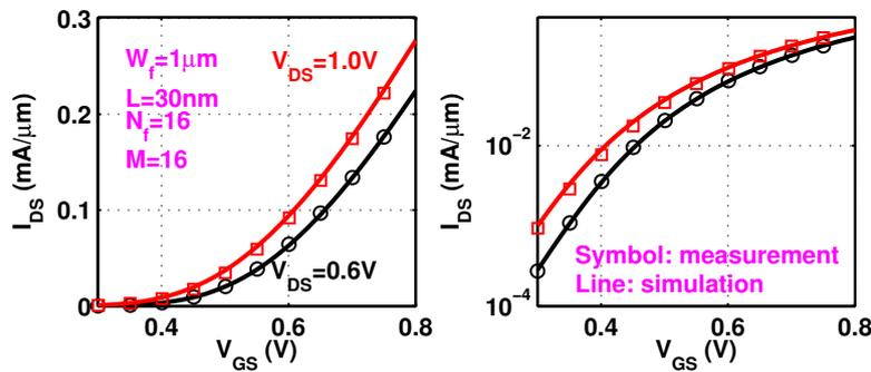
**Figure 5.** Comparison of simulated  $I_{DS}$  versus  $V_{GS}$  with measurement on (a) linear and (b) log  $I_{DS}$  scales at  $V_{DS} = 0.6$  and  $1.0$  V.
