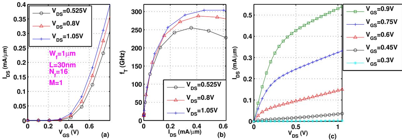
Figure 1. Measured (a)  $I_{DS}$  versus  $V_{GS}$ ; (b)  $f_T$  versus  $I_{DS}$  and (c)  $I_{DS}$  versus  $V_{DS}$ .
