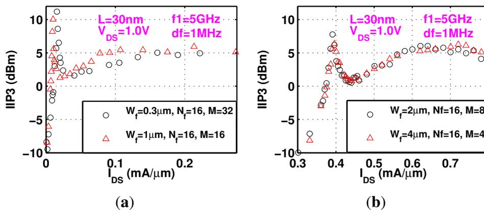
**Figure 8.** Measured width impact on  $IIP3$ . (a) Measured  $IIP3$  at 5 GHz for two 30 nm devices with different total width; (b) Measured  $IIP3$  as a function of  $V_{GS}$  for two 30 nm devices with same total width.
