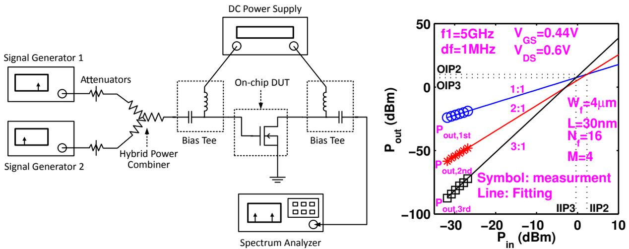
Figure 2. (a) Measurement setup and (b) extrapolation illustration for  $IP3$  and  $IP2$ .
