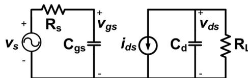
**Figure 3.** Simplified equivalent circuit used for  $IIP3$  derivation using Volterra series.
