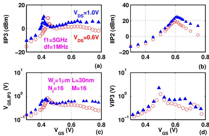
**Figure 7.** Measured (a)  $IIP3$ ; (b)  $IIP2$  and (c)  $V_{GS,IP3}$  and (d)  $VIP3$  as a function of  $V_{GS}$  for different  $V_{DS}$ .
