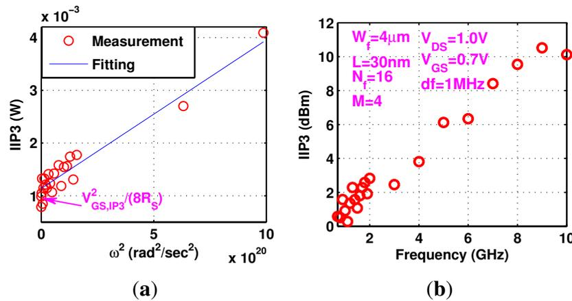
**Figure 4.** Frequency dependence of  $IIP3$  at  $V_{GS} = 0.7$  V and  $V_{DS} = 1.0$  V. (a) Measured  $IIP3$  in watt versus  $\omega^2$ ; (b) Measured  $IIP3$  in dBm versus frequency.
