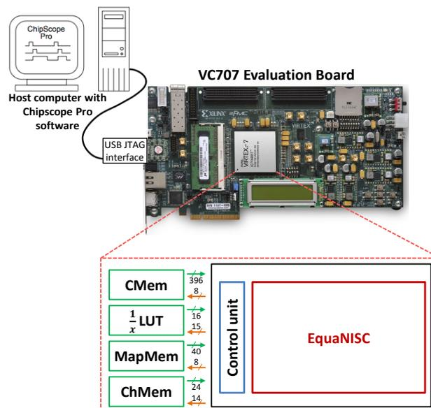
Figure 13. NISC-based MMSE MIMO turbo equalizer architecture on-chip prototype.
