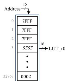
Figure 12.  $\frac{1}{x}$  LUT structure.
