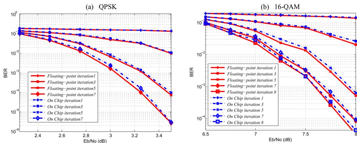
**Figure 16.** Comparison between the simulated reference BER and measured BER after on-chip evaluation of the designed equalizer for 1536 source bits, a  $\frac{1}{2}$  code rate,  $4 \times 4$  MIMO and a fast fading Rayleigh channel.
