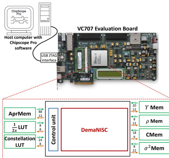
Figure 15. NISC-based demapper architecture on-chip prototype.
