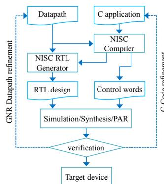
Figure 6. NISC tool set generic design flow.
