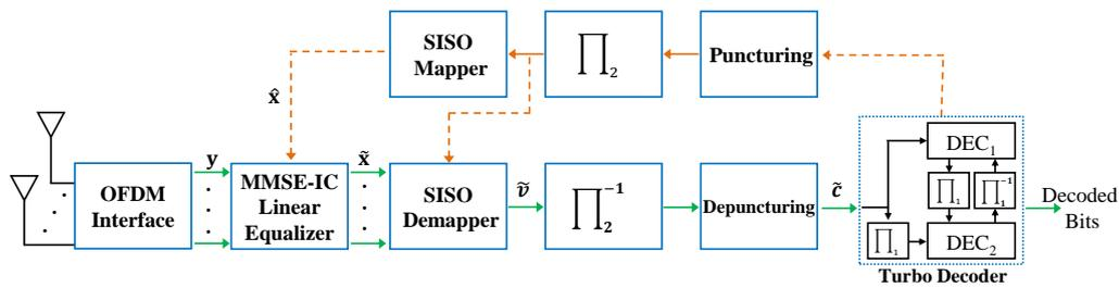
Figure 1. Block diagram of the MIMO-OFDM turbo receiver.
