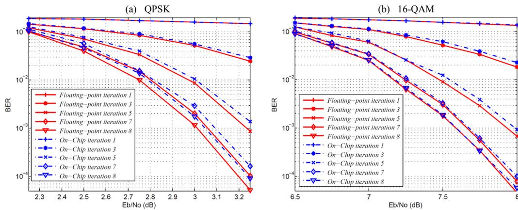
**Figure 17.** Comparison between the simulated reference BER and measured BER after on-chip evaluation of the designed demapper for for 1536 source bits, a  $\frac{1}{2}$  code rate,  $4 \times 4$  MIMO and fast fading Rayleigh channel.
