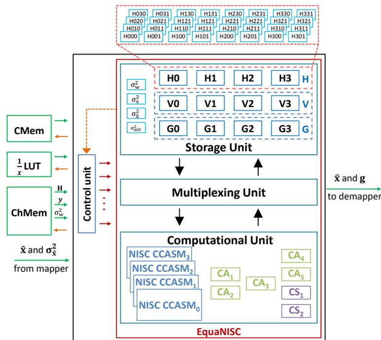
Figure 3. Proposed equalizer architecture.
