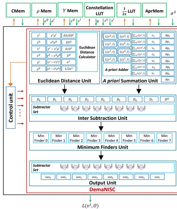
Figure 4. Proposed NISC-based demapper architecture.
