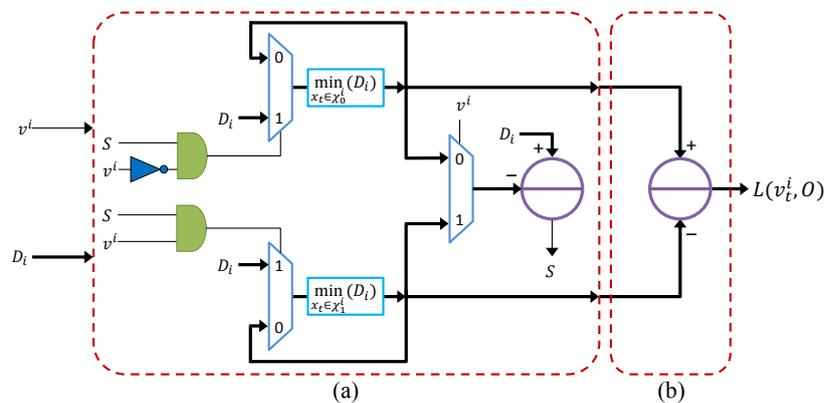
**Figure 5.** (a) Minimum finder operational unit; (b) subtractor used in the subtraction operation of the minimum pair.
