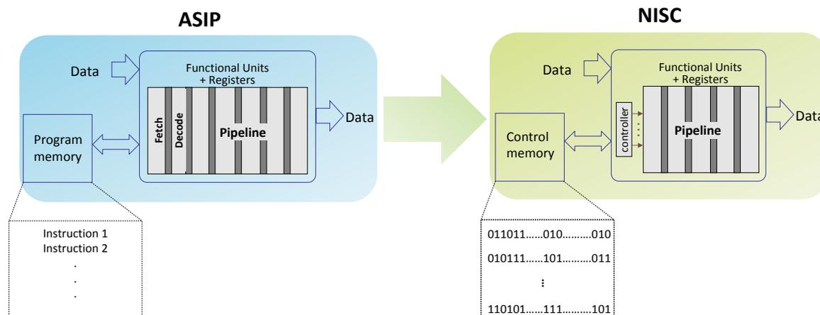
**Figure 2.** Transition from the application-specific instruction set processor (ASIP) to the no instruction set computer (NISC) design approach.
