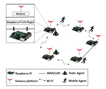
Figure 2. Top level architecture of AgPi (Agents on Pi).
