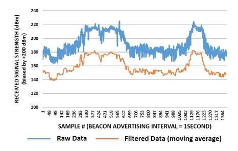
Figure 7. BLE raw and filtered data.
