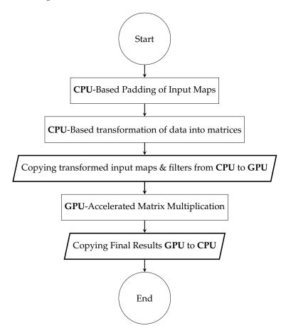
Figure 8. Flow of CPU padded ConvMM.
