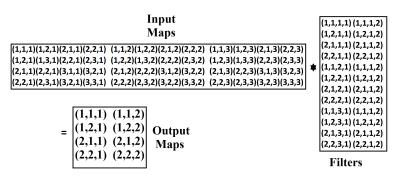
Figure 3. Convolution matrix multiplication.
