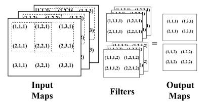
Figure 2. Three-dimensional convolution layer.
