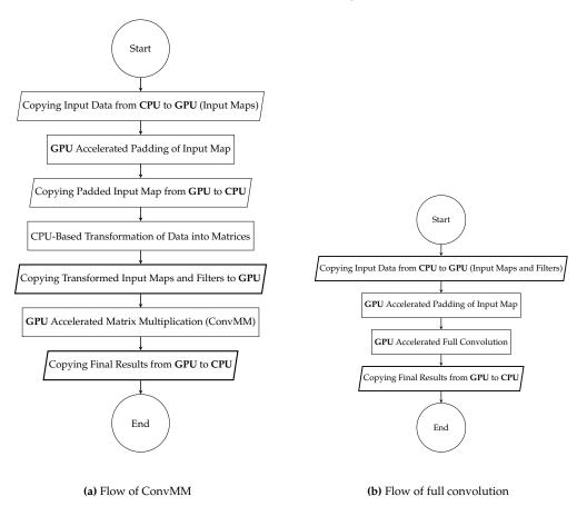
Figure 5. Flow of ConvMM and full convolution.
