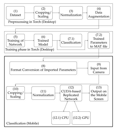
Figure 1. Block diagram of the mobile platform-based deep classifier.
