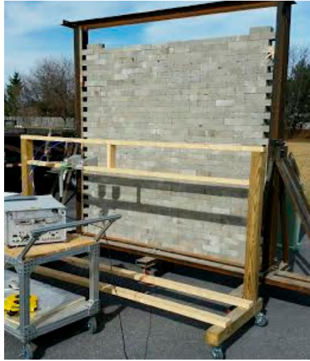
Figure 3. Photograph showing the cart with the horn antennas mounted and the wall behind which the targets were located.
