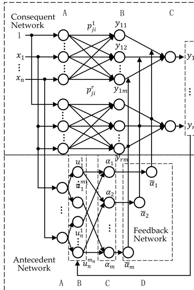
Figure 3. Structure of T-S fuzzy neural network (TSFNN).
