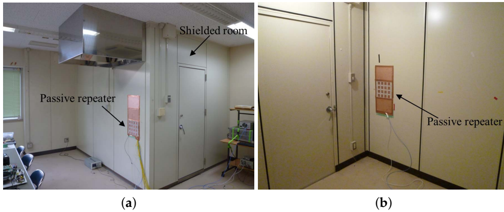
Figure 12. The shielded room. (a) Outline of shielded room; (b) Inside view of shielded room.
