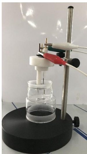
Figure S1. Digital photo of the electrochemical cell used in this work.
