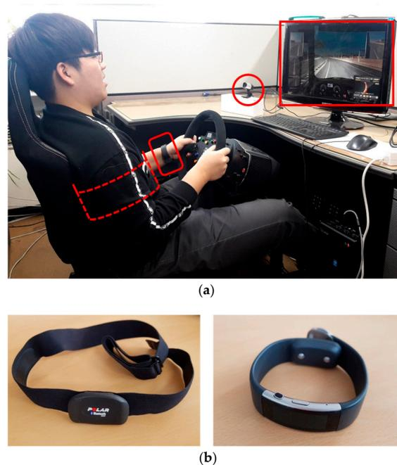
**Figure 2.** Data collection instruments and environment: (a) Driving simulation environment; (b) physiological devices used for heart rate variability (HRV) collection: POLAR H7 Strap (left) and Microsoft BAND 2 (right).
