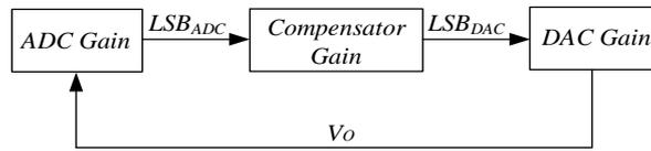
Figure 2. Digital closed-loop system block diagram.
