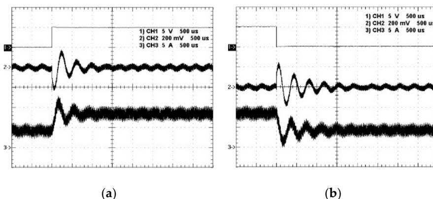
**Figure 13.** Waveforms based on the traditional PWM control strategy: (1) load enable; (2) AC output voltage; (3) inductor current, due to (a) from 50% to 100%; (b) from 100% to 50%.
