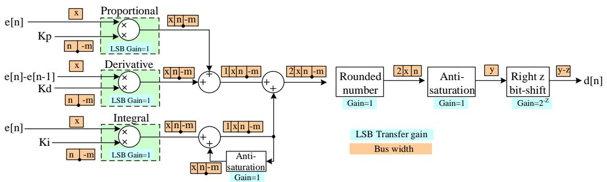
Figure 7. Proportional–integral–derivative (PID) compensator block diagram.
