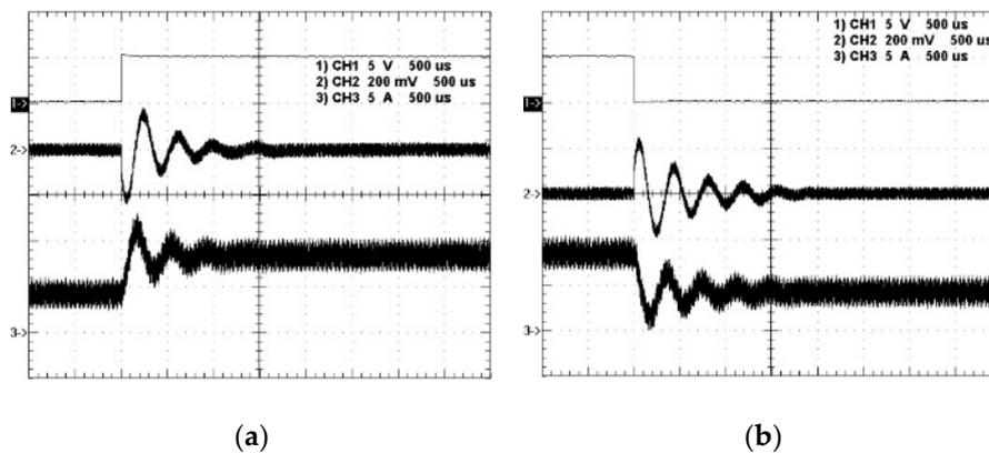
**Figure 15.** Waveforms based on the proposed PWFM control strategy: (1) load enable; (2) AC output voltage; (3) inductor current, due to (a) from 50% to 100%; (b) from 100% to 50%.
