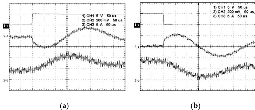
**Figure 17.** Zoom-in waveforms based on the traditional PWM control strategy: (1) load enable; (2) AC output voltage; (3) inductor current, due to (a) from 50% to 100%; (b) from 100% to 50%.
