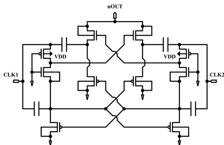
Figure 4. Proposed enhanced clock pump circuit (ECPC).
