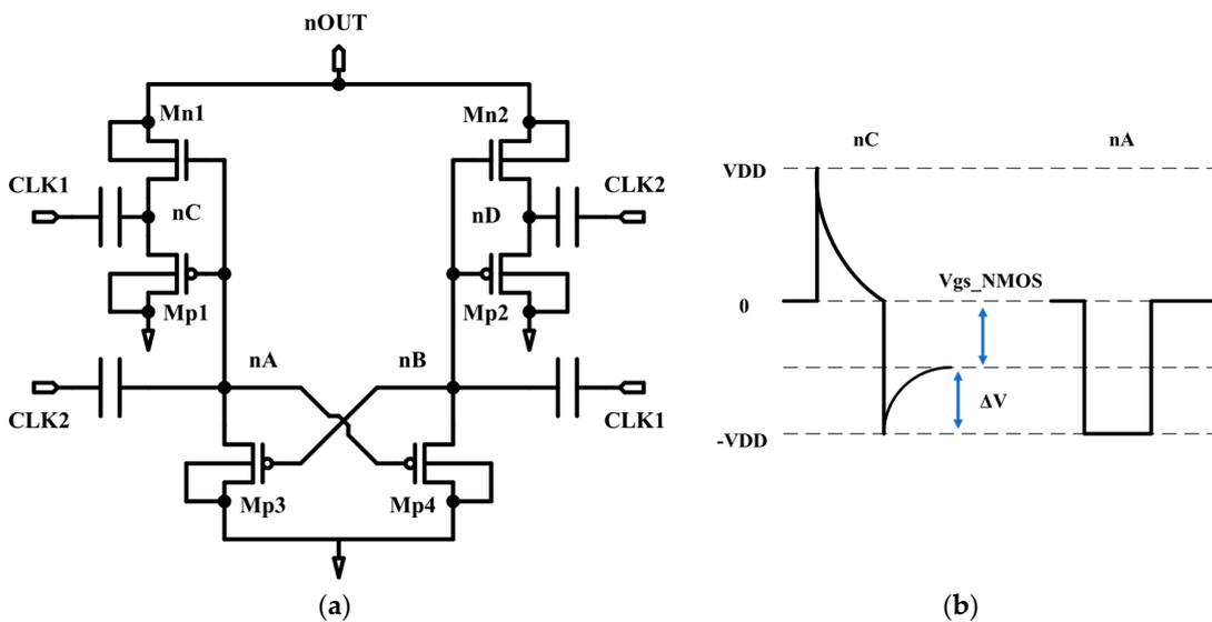
**Figure 3.** (a) Cross-coupled hybrid pump circuit 2 (CHPC2) and (b) its voltage waveforms at pumping nodes during the initial pump down operation.
