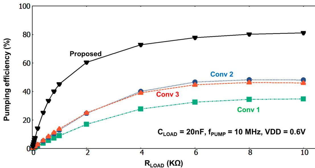
Figure 10. Pumping efficiency with various load resistance at  $V_{DD} = 0.6\text{ V}$ .
