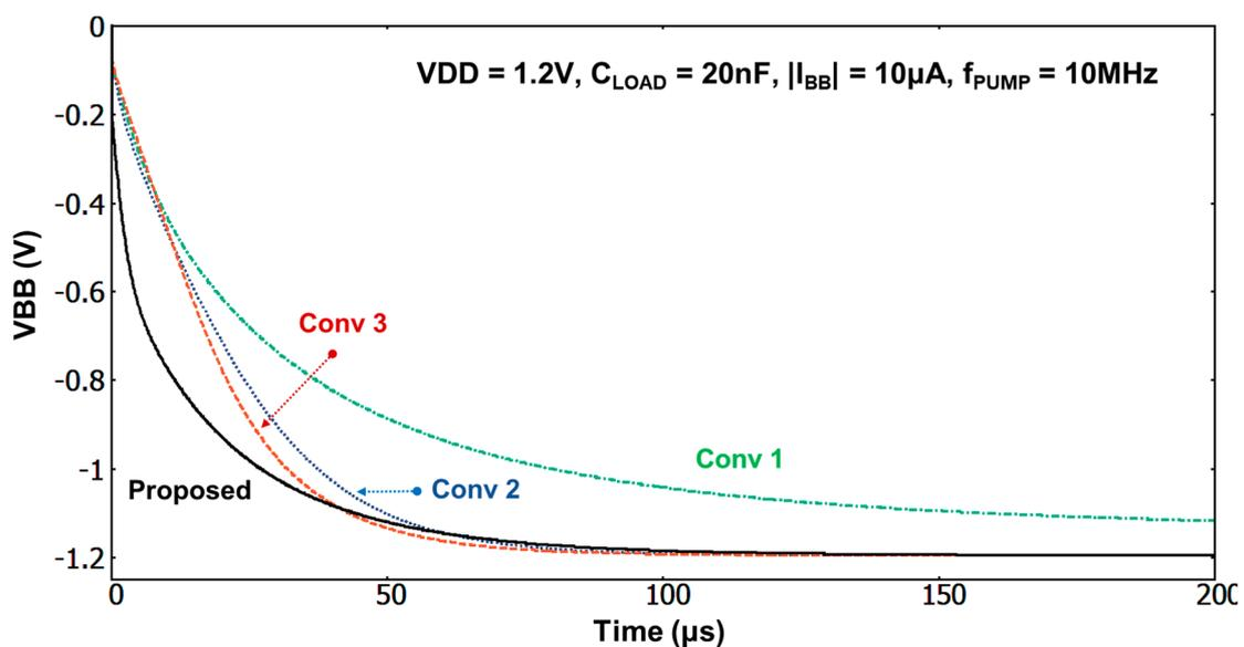
Figure 6. Comparison of the pump down speeds.
