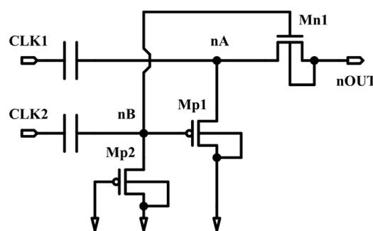
**Figure 1.** The schematic diagram of hybrid pumping circuit (HPC).
