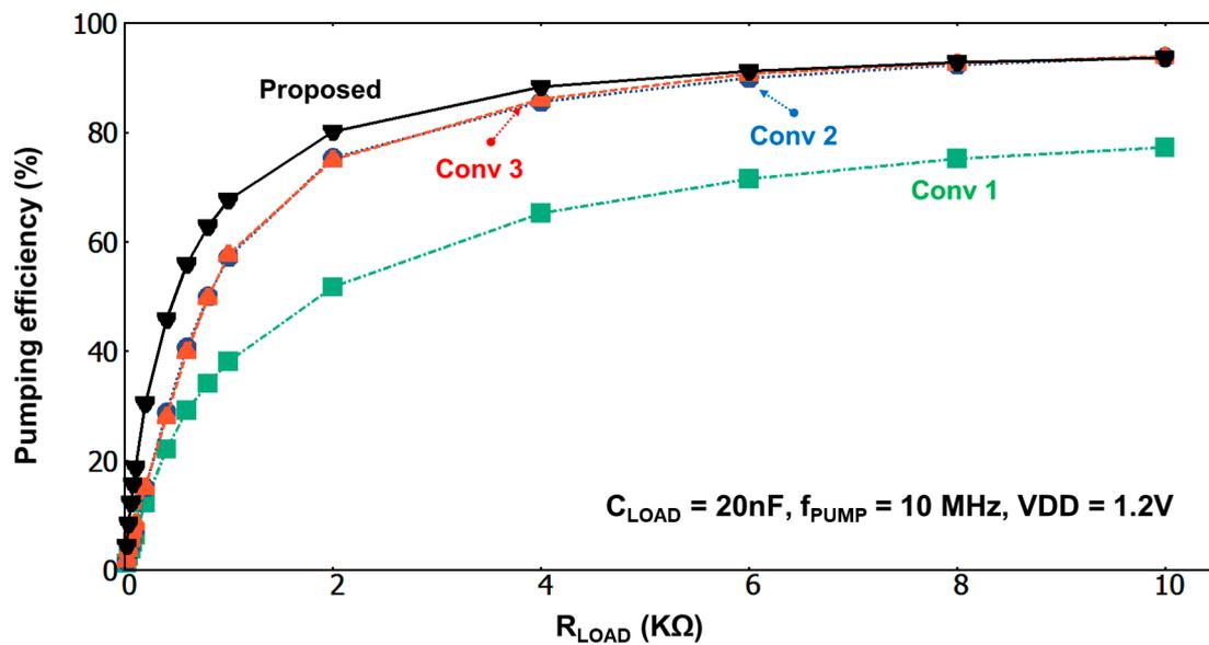
Figure 9. Pumping efficiency with various load resistance at  $V_{DD} = 1.2$  V.
