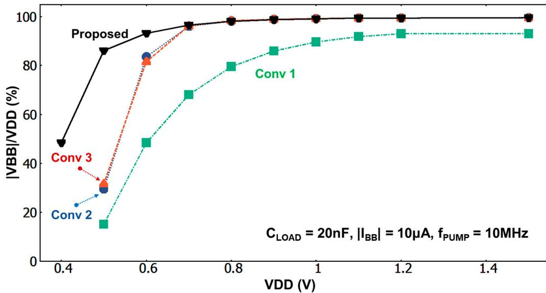
Figure 7.  $|V_{BB}|/V_{DD}$  with various supply voltages.
