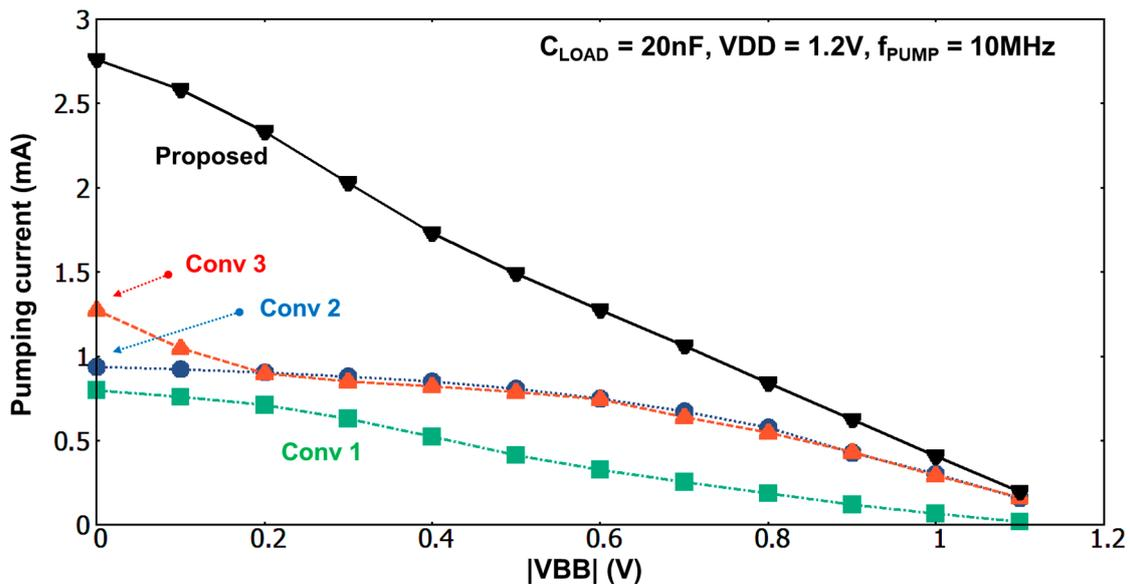
Figure 8. Pumping current with various  $V_{BB}$ .
