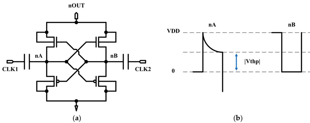
**Figure 2.** (a) Cross-coupled hybrid pump circuit 1 (CHPC1) and (b) its voltage waveforms at pumping nodes during the initial pump down operation.
